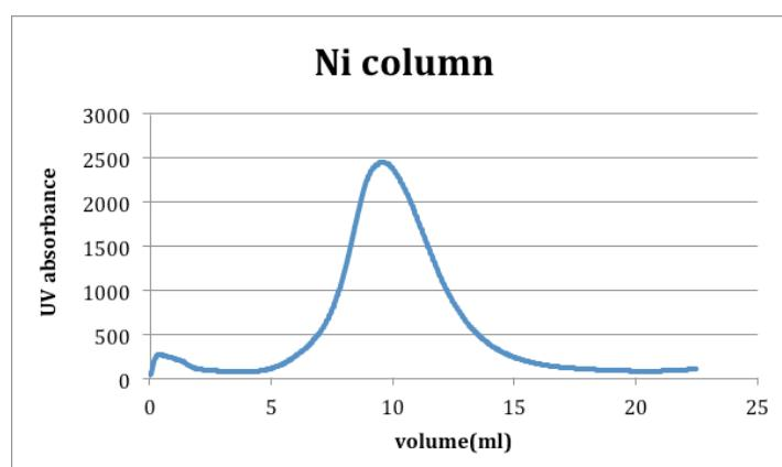
FPLC Chart for Ni column purification using AKTA machine
