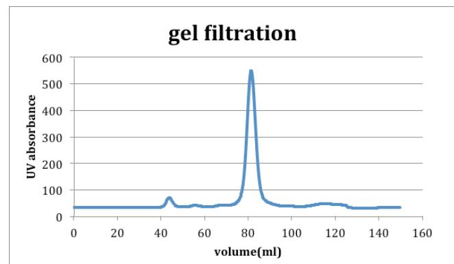
FPLC Chart for S200 column purification using AKTA machine
