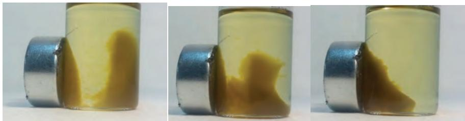
**Figure S118.** Sequential pictures of the attraction by a magnet of nanospheres of poly(**1<sub>0.2</sub>-co-7<sub>0.8</sub>**) incorporating magnetic nanoparticles.
