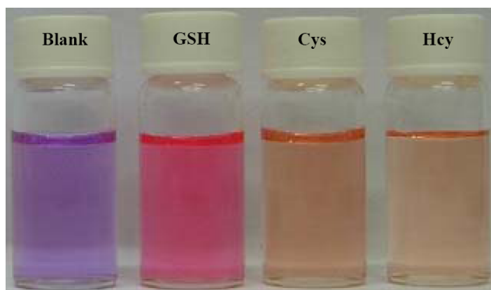
Figure S13. Color changes of the solution of probe 1 (8 \mu\text{M} ) with the addition of 10 equiv of Cys, Hcy and GSH in DMF/phosphate buffer (3:7 v/v, 20 mM, pH 7.4) for 10 min.
