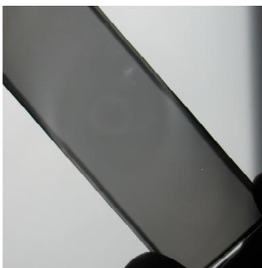
Fig. S11 Photograph of spin coated SnTe film on borosilicate glass.
