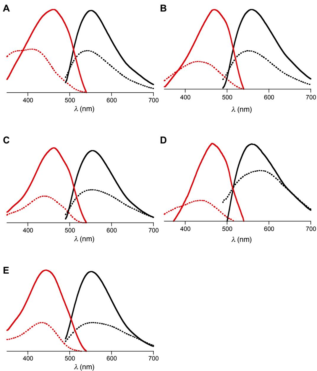
**Figure S1.** Excitation (red,  $\lambda_{\text{em}} = 560$  nm) and emission spectra (black,  $\lambda_{\text{ex}} = 430$  nm) of probes (A) **8**, (B) **9**, (C) **10**, (D) **11** and (E) **13** in DPPC (solid) and DOPC (dotted) LUVs at 25 °C.
