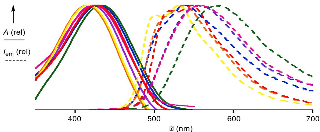
**Figure S3.** Normalized absorption (solid) and emission (dotted) spectra of **77** in, with increasingly red-shifted emission, hexane (yellow), diethyl ether (orange), toluene (red), THF (magenta), acetone (purple), DMF (blue), DMSO (dark green).
