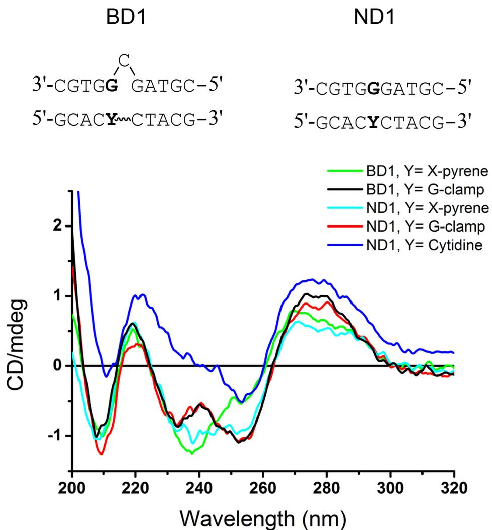
**Figure S19.** CD spectra of bulge duplex and normal duplexes (Y = X-pyrene, G-clamp or C) were recorded from 200 nm to 320 nm. The signals were smoothed by Savitzky-Golay method (20 pts, polynomial order = 2) in Origin 8.6 software.
