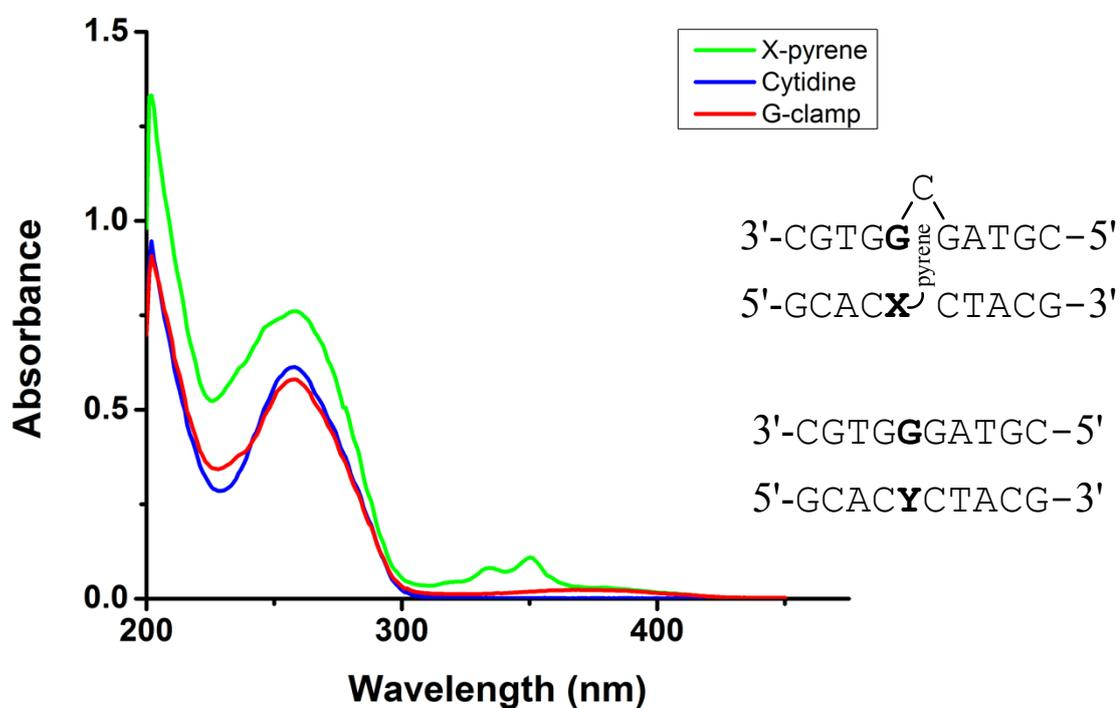
**Figure S9:** Representative UV absorption curves of ND1 (Y = G-clamp or C, 2.5  $\mu$ M) and X-pyrene bulged duplex (BD1, 2.5  $\mu$ M) within the range of 200 - 475 nm: BD1 is in green, ND1 containing G-clamp in red and ND1 containing C in blue.
