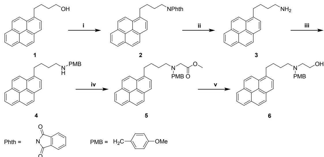
**Scheme S1.** Reagents and conditions: (i) phthalimide,  $\text{PPh}_3$ , DEAD, THF, RT, 1 h; (ii)  $\text{H}_2\text{NNH}_2 \cdot \text{H}_2\text{O}$ , EtOH/DCM (1:1), RT, 72 h, 87 % for two steps from **1** to **3**; (iii) 4-methoxybenzyl chloride, NaH, DMF, 0 °C, 24 h, 43 %; (iv) methyl bromoacetate, NaH, DMF, 0 °C, 1 h; (v)  $\text{LiBH}_4$ , THF, RT, 72 h, 49 % for two steps from **4** to **6**.
