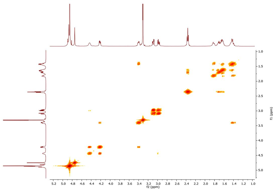
**Figure S3:** 2D-NMR (500 MHz, MeOD-d<sub>4</sub>) COSY: Biotin[6]juril-hexamethylester-D<sub>18</sub>.
