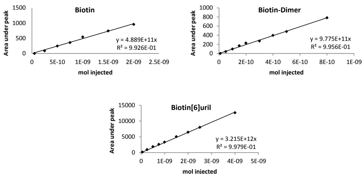
**Figure S62:** Standard curves at 209 nm of Biotin, Biotin-dimer, and Biotin[6]uril.
