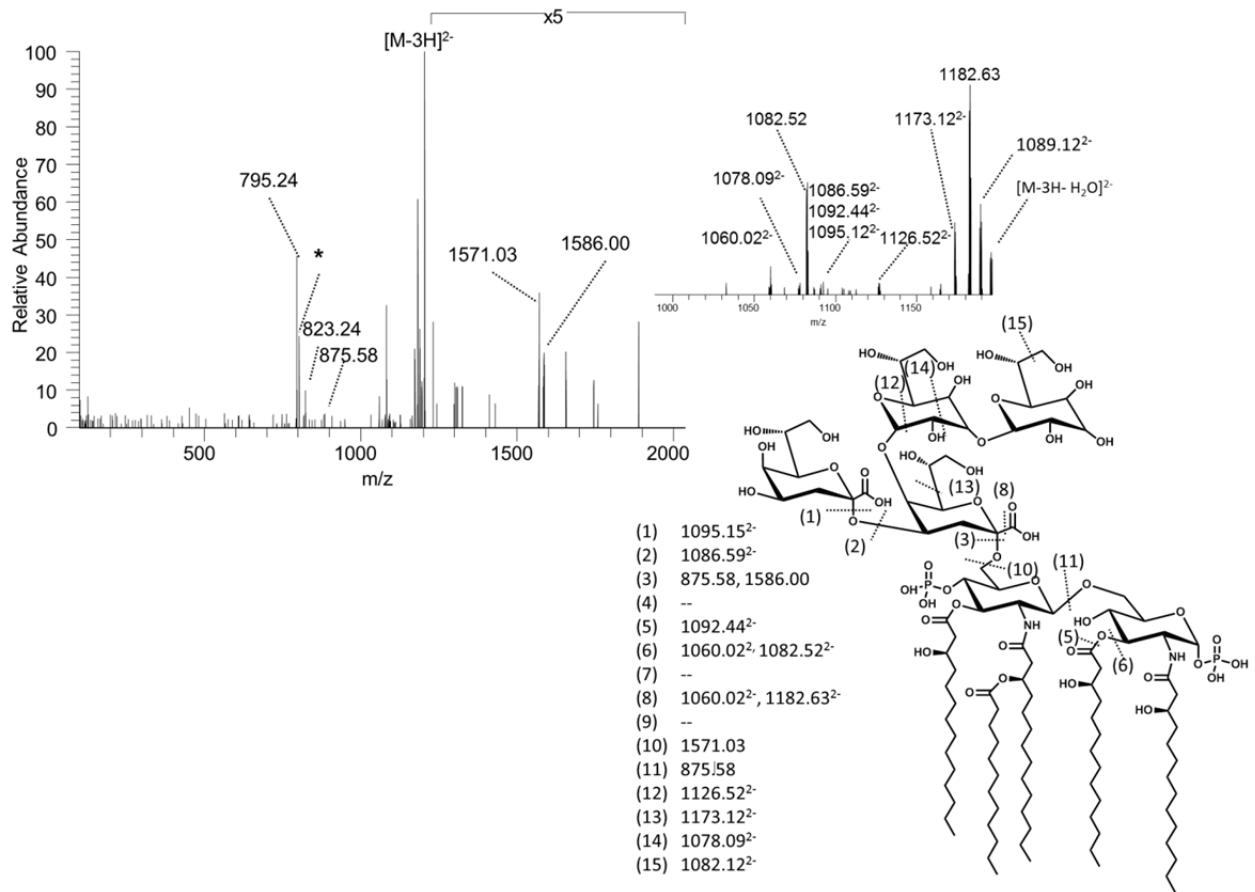
**Figure S12.** UVPD mass spectrum of penta-acyl waaQwaaG ( $z = 3$ ) [ $\text{Mr} = 2411.27$ ] from BN1  $\Delta$ waaQwaaG. The corresponding fragmentation map is shown on the right.
