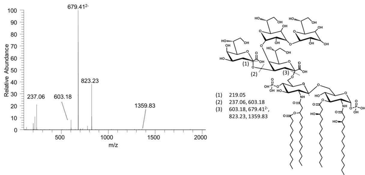
**Figure S9.** HCD mass spectrum of tetra-acyl waaQwaaG ( $z = 3^-$ ) [ $\text{Mr} = 2185.07$ ] from BN1  $\Delta$ waaQwaaG. The corresponding fragmentation map is shown on the right.
