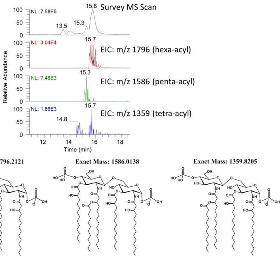
**Figure S13:** LC-MS trace and extracted ion chromatograms of the UVPD/HCD fragment ions associated with the identified BN1 LOS lipid A anchors . The structures of the different fragment ions are shown below.
