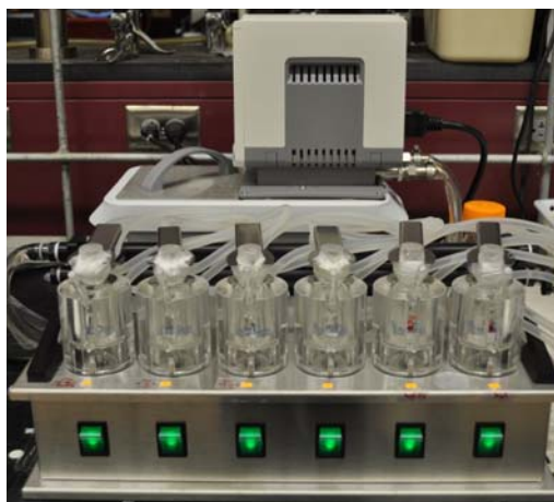
Fig. S1 Picture of the diffusion system with six-station vertical cell stirrers.
