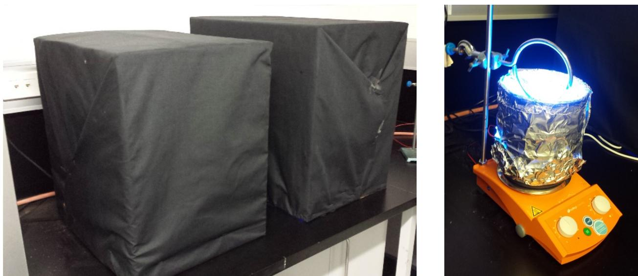
**Figure S1.** Experimental setup for photo-polymerization using 4.8 Watts blue LED light.
