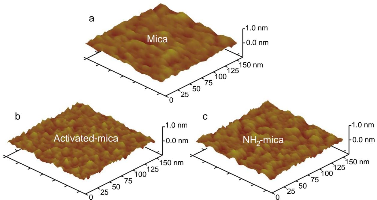
**Fig. S2** AFM images of (a) cleaved mica, (b) activated mica, and (c) monolayer APTES-modified mica.
