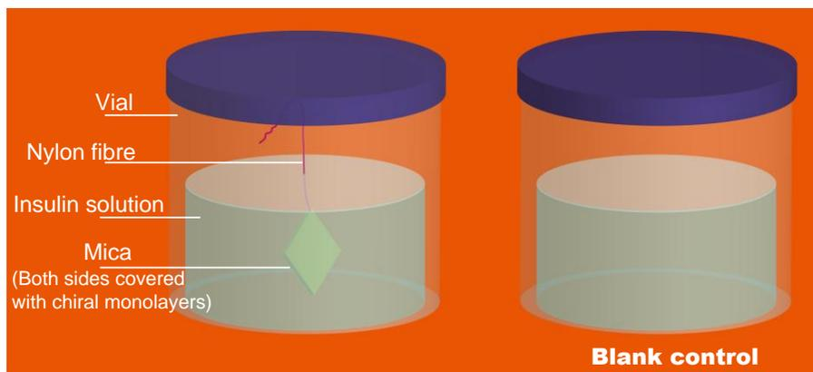
**Fig. S5** Schematic showing the quantitative determination method of the chiral surfaces-adsorbed insulin. Although only one mica wafer was shown in the figure, 10 mica wafers were simultaneously suspended for better accuracy in real determinations. Five parallel samples were carried out for each determination.
