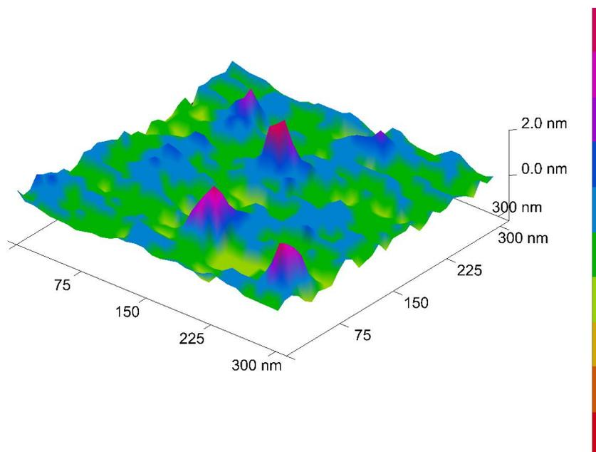
**Fig. S3** Magnified AFM image of the tiny dots with height of 1-2 nm.
