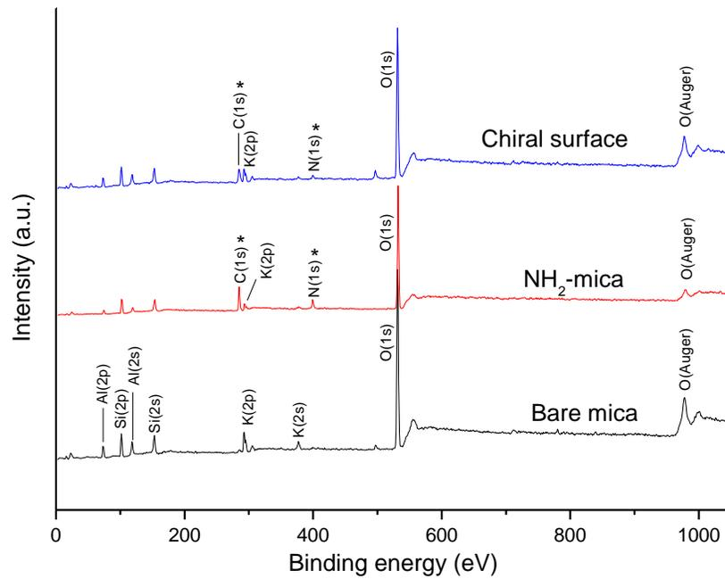
**Fig. S1** XPS surveys of D-surface (blue), NH<sub>2</sub>-mica (red) and bare mica (black).
