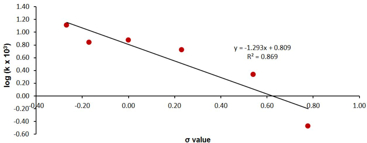
**Figure S7.** Hammett plot of rate constants from reactions of DNICs (**1a-1e, 1**) with CO.
