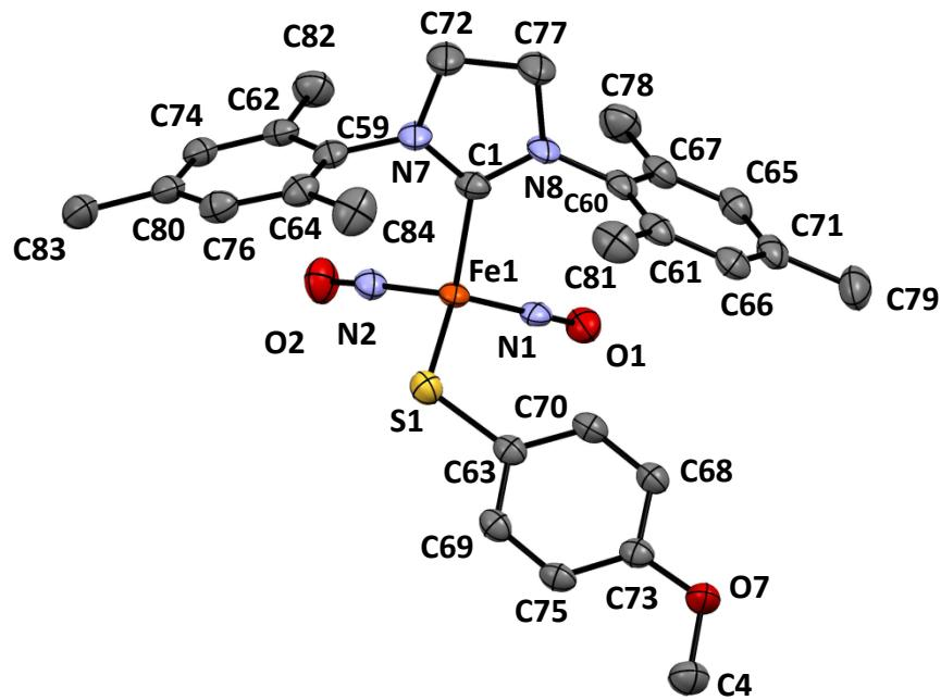
**Figure S1a.** ORTEP drawing and labeling scheme of complex **1a** with thermal ellipsoids drawn at 50% probability. Hydrogen atoms are omitted for clarity.
