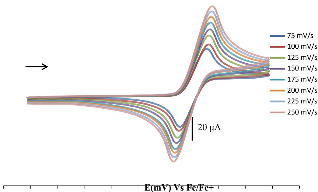
**Figure S6.** Scan rate – independent reversibility of **1b** (THF solution, scan rates 75-250 mV/s) as representative of DNICs **1**, **1a-1e**
