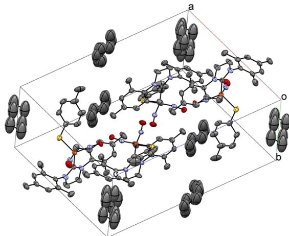
**Figure S2b.** Unit cell of complex **1b** complete with 4 cyclohexane molecules of crystallization.\*
