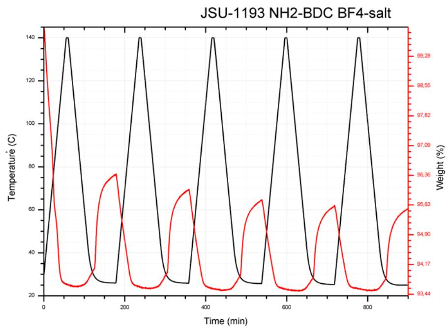
**Figure S10.** Temperature dependent cycling of reversible O<sub>2</sub> binding by **2b**(BF<sub>4</sub>)<sub>4</sub> measured using TGA.
