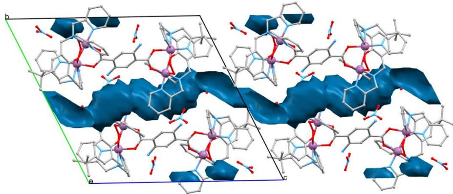
**Figure S6.** View of **2b**(NO<sub>3</sub>)<sub>4</sub> (lattice water removed *in silico*) down the *a*-axis showing voids running parallel to the *b*-axis. Void calculation was performed in Mercury CSD 3.3.1 with a probe radius of 1.2 Å and grid spacing 0.7 Å resulting in a volume of 200.18 Å<sup>3</sup> / 4.8% per unit cell
