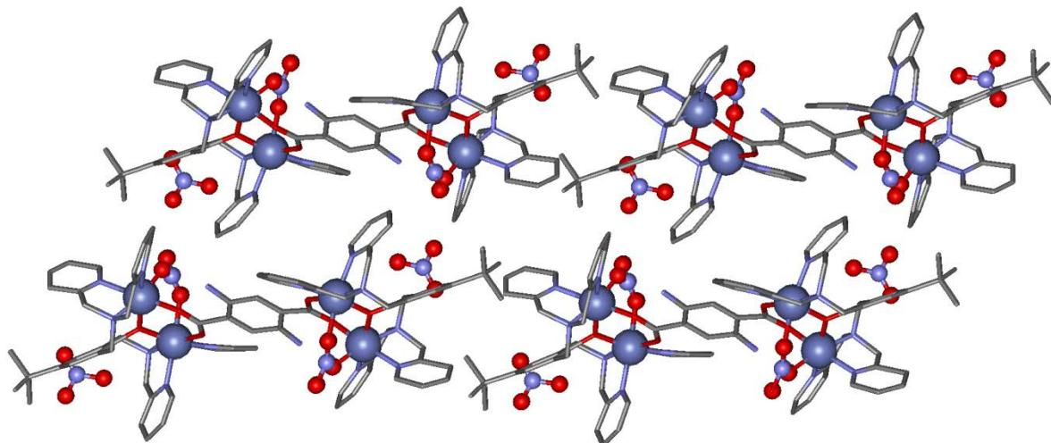
**Figure S1(c)** Illustration of deoxygenated structure, viewed down the *b* axis. Selected atoms are shown as balls to illustrate aspects of the structure (Co = large blue balls, N = small blue balls, O = red balls). Carbon atoms are shown as vertices, while hydrogen atoms and solvent molecules are omitted for clarity.
