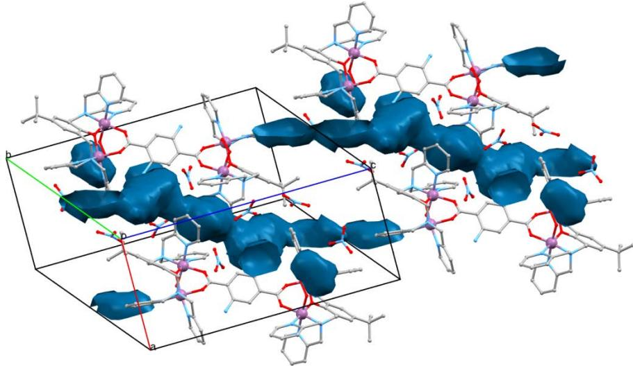
**Figure S8.** Perspective view the voids in of  $\mathbf{2b}(\text{NO}_3)_4$  (lattice water removed *in silico*).
