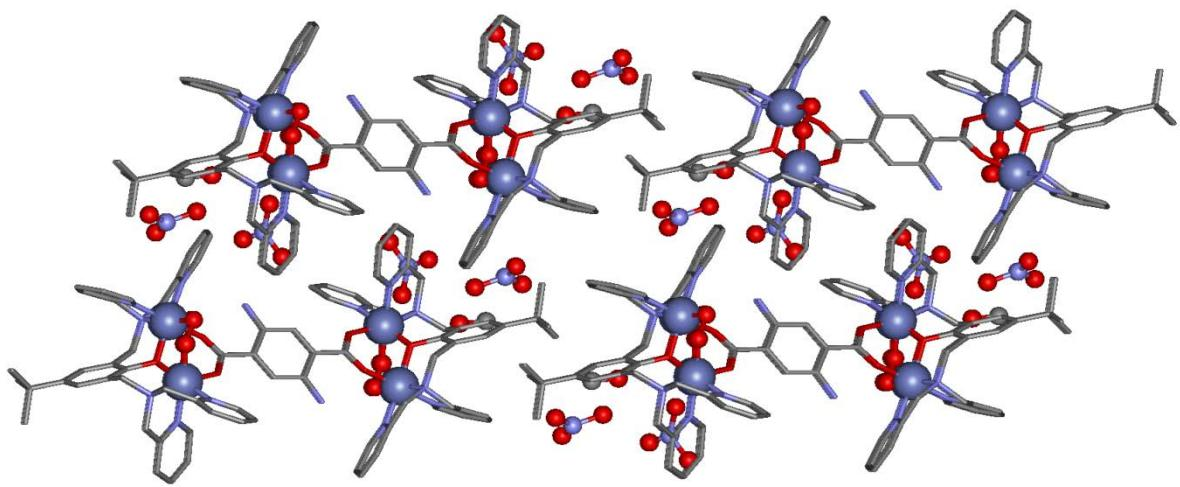
**Figure S1(b)** Illustration of oxygenated structure, viewed down the *b* axis. Selected atoms are shown as balls to illustrate aspects of the structure (Co = large blue balls, N = small blue balls, O = red balls). Carbon atoms are shown as vertices, while hydrogen atoms and solvent molecules are omitted for clarity.
