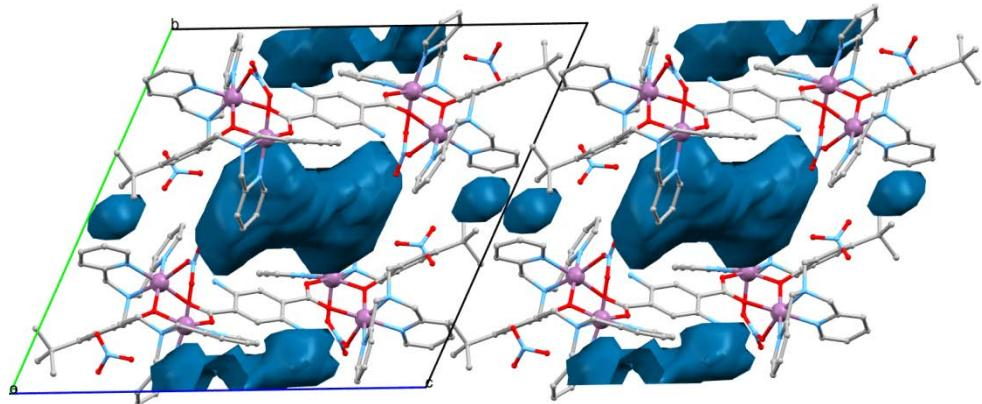
**Figure S7.** View of **2b**<sub>deoxy</sub>(NO<sub>3</sub>)<sub>4</sub> (lattice water removed *in silico*) down the *a*-axis showing how the voids running parallel to the *b*-axis become disconnected. Void calculation was performed in Mercury CSD 3.3.1 with a probe radius of 1.2 Å and grid spacing 0.7 Å resulting in a volume of 300.99 Å<sup>3</sup> / 7.0% per unit cell
