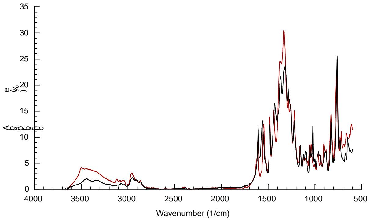
**Figure S3.** IR spectra of **2b**(NO<sub>4</sub>)<sub>4</sub>•7H<sub>2</sub>O at -20 °C (red) and 120 °C (black) showing reduction in intensity of the broad band at 3000 to 3500  $\text{cm}^{-1}$  attributed to loss of water.
