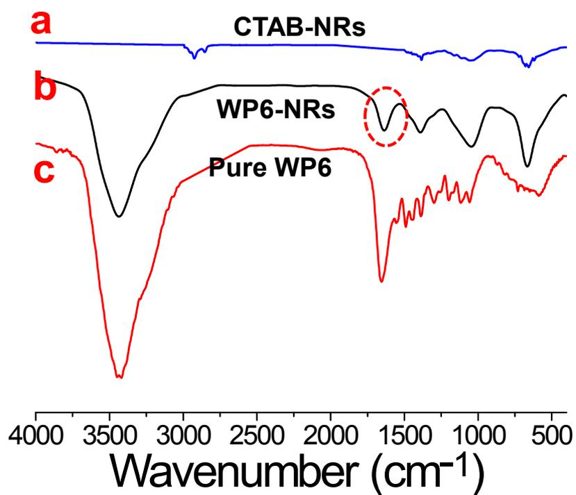
**Fig. S18.** Fourier transform IR spectra: (a) CTAB stabilized NRs; (b) **WP6** stabilized NRs; (c) pure **WP6**. The circle indicates the C=C stretching mode of the benzene ring.
