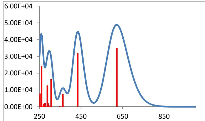
**Fig. S7.** Calculated (B3LYP/6-31G\*) absorption spectrum of **S2-Ph**.
