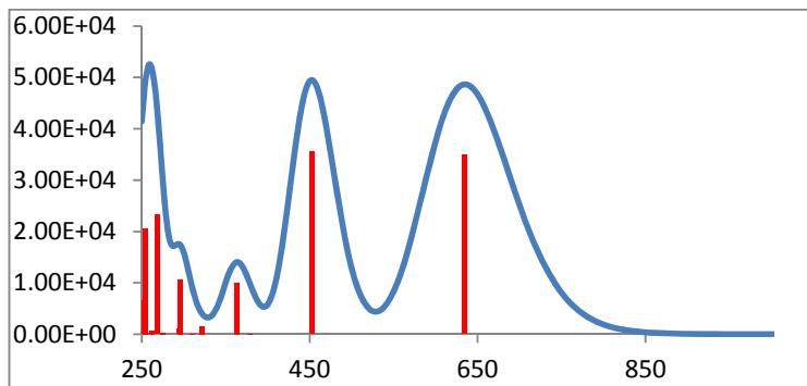
**Fig. S5.** Calculated (B3LYP/6-31G\*) absorption spectrum of **S2-TIPS**.
