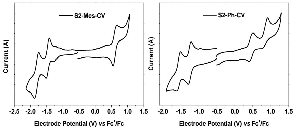
**Fig. S14.** Cyclic voltammograms of S2-Mes and S2-Ph in dry dichloromethane containing 0.1 M Bu<sub>4</sub>NPF<sub>6</sub> as the supporting electrolyte, AgCl/Ag as the reference electrode, Au as the working electrode, Pt wire as the counter electrode, and a scan rate of 50 mV s<sup>-1</sup>. The potential was externally calibrated against the ferrocene/ferrocenium couple.
