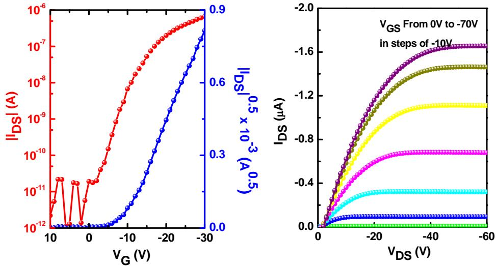
**Fig. S11.** Transfer and output characteristics of FET devices fabricated by solution casting of **S2-TIPS** on OTS-treated substrates when operated in N<sub>2</sub>.
