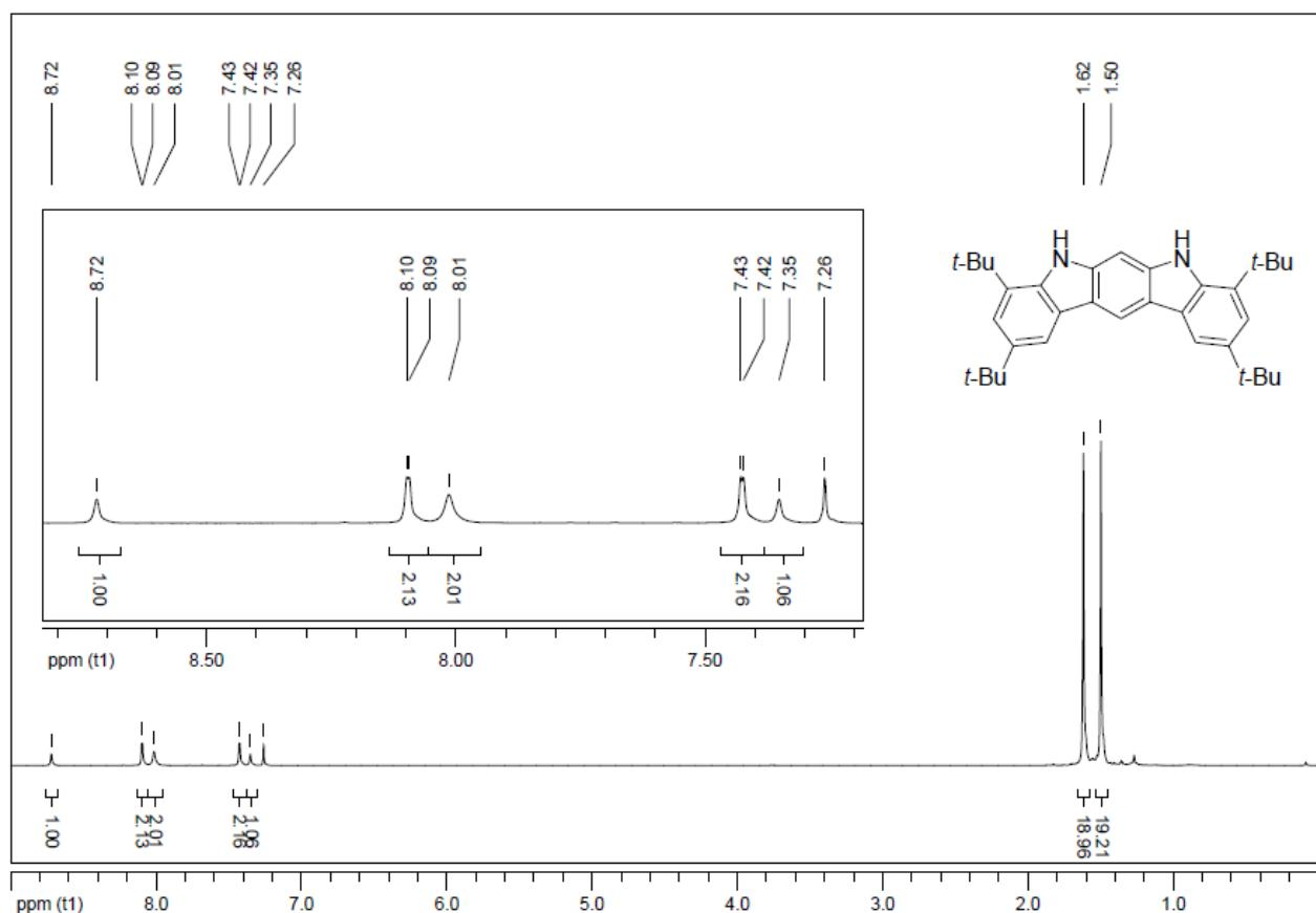
**Fig. S16.**  $^1\text{H}$  NMR spectrum of compound **6** ( $\text{CDCl}_3$ , 300 MHz, rt).
