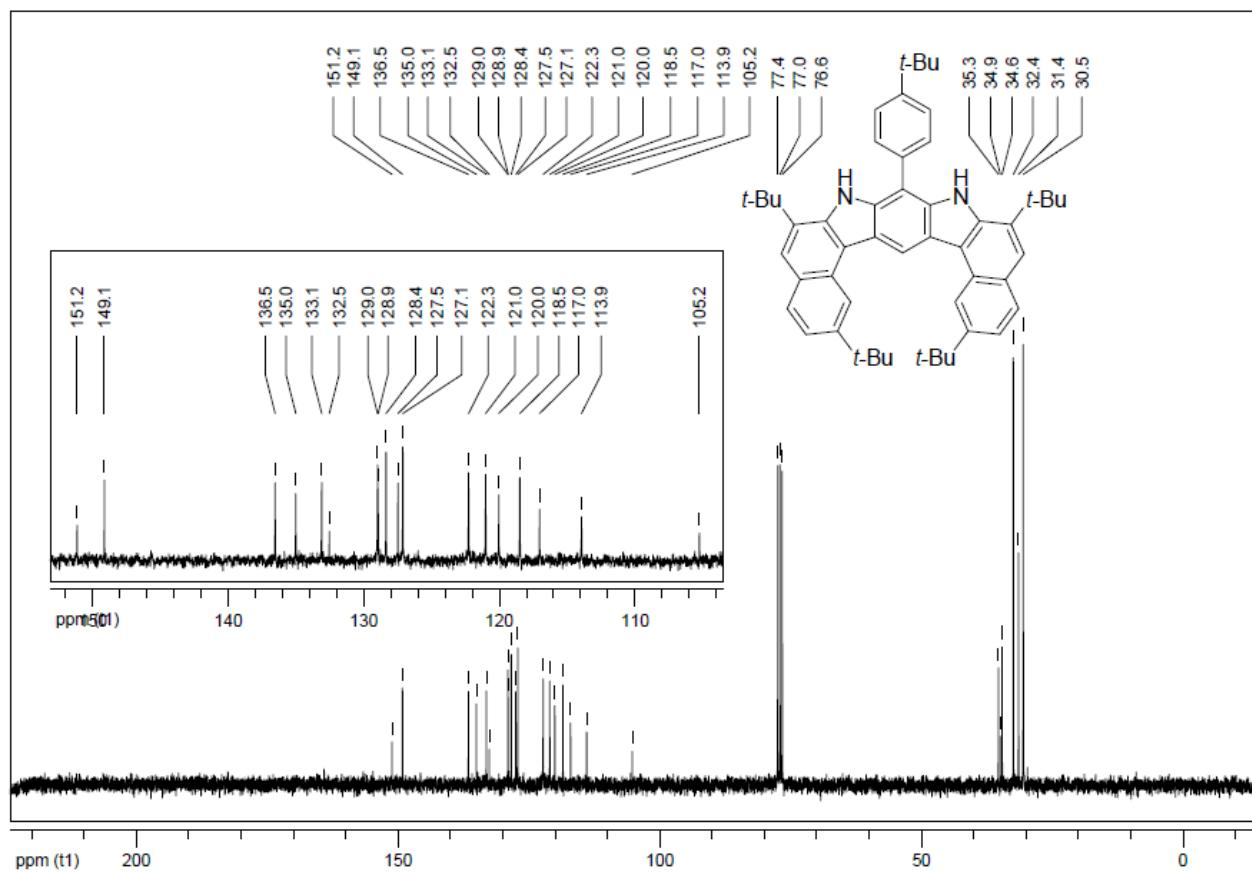
**Fig. S35.**  $^{13}\text{C}$  NMR spectrum of compound **15** ( $\text{CDCl}_3$ , 75 MHz, rt).
