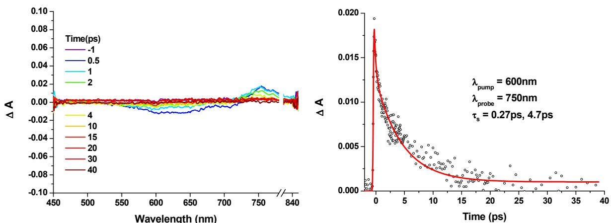
**Fig. S3.** Transient absorption spectrum and decay curve of **2** in toluene.
