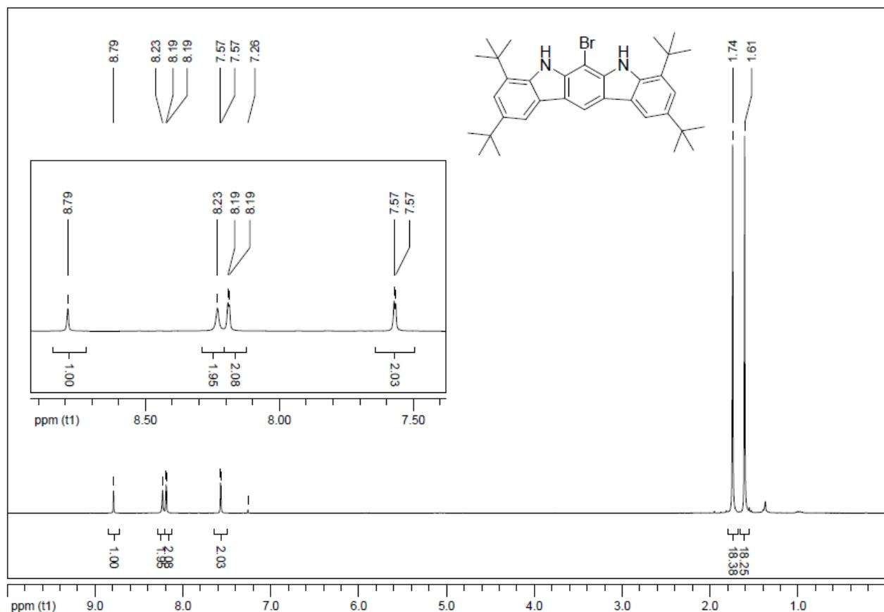
**Fig. S19.**  $^1\text{H}$  NMR spectrum of compound 7 ( $\text{CDCl}_3$ , 300 MHz, rt).
