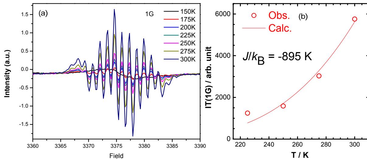
**Fig. S1.** (a) VT ESR spectra of the freshly prepared solution of **1** upon warm up from 150K to 300K (modulation amplitude of 1 G). (b) Fitting of the VT ESR data by Bleaney-Bowers equation. Due to uncertainty of the ESR intensity change at about 150 K (melting point of 2-Me THF), only the data above 200 K was used for simulation.
