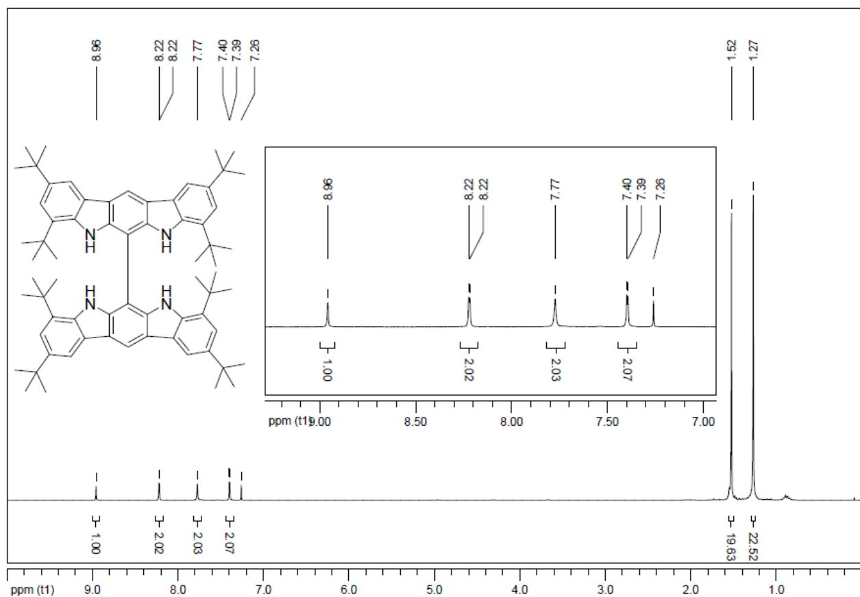
**Fig. S40.**  $^1\text{H}$  NMR spectrum of compound **16** ( $\text{CDCl}_3$ , 300 MHz, rt).
