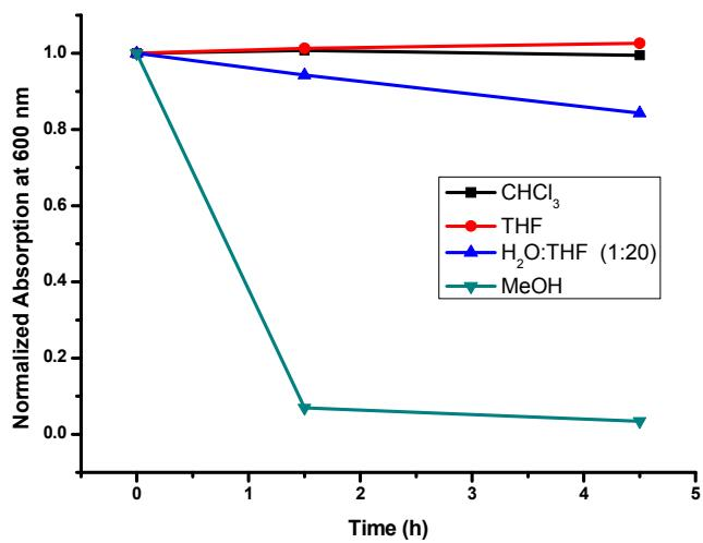
**Fig. S6.** The decay of **2** in different solvents indicated by the optical density at 600 nm vs time.
