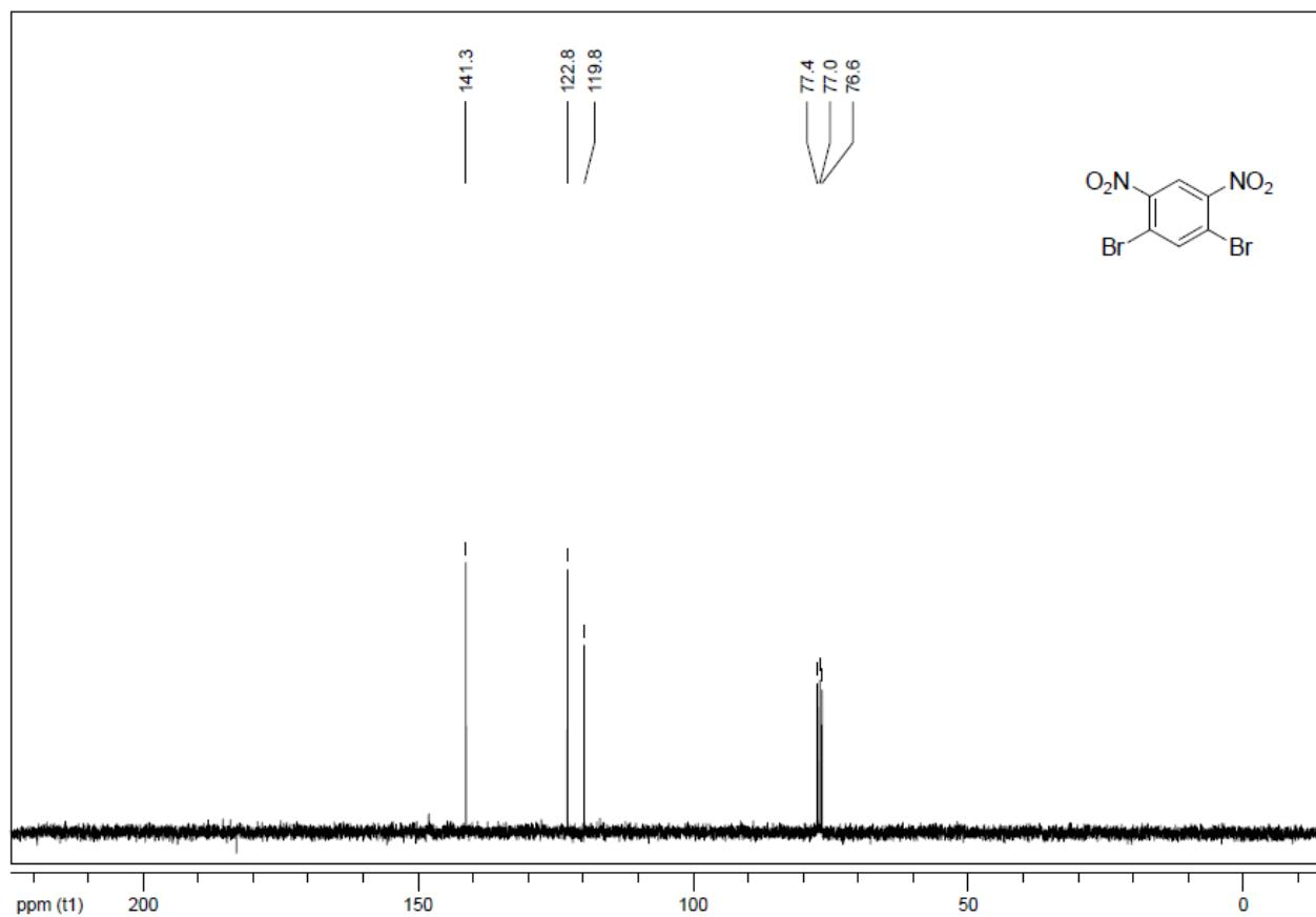
**Fig. S11.**  $^{13}\text{C}$  NMR spectrum of compound 4 ( $\text{CDCl}_3$ , 75 MHz, rt).
