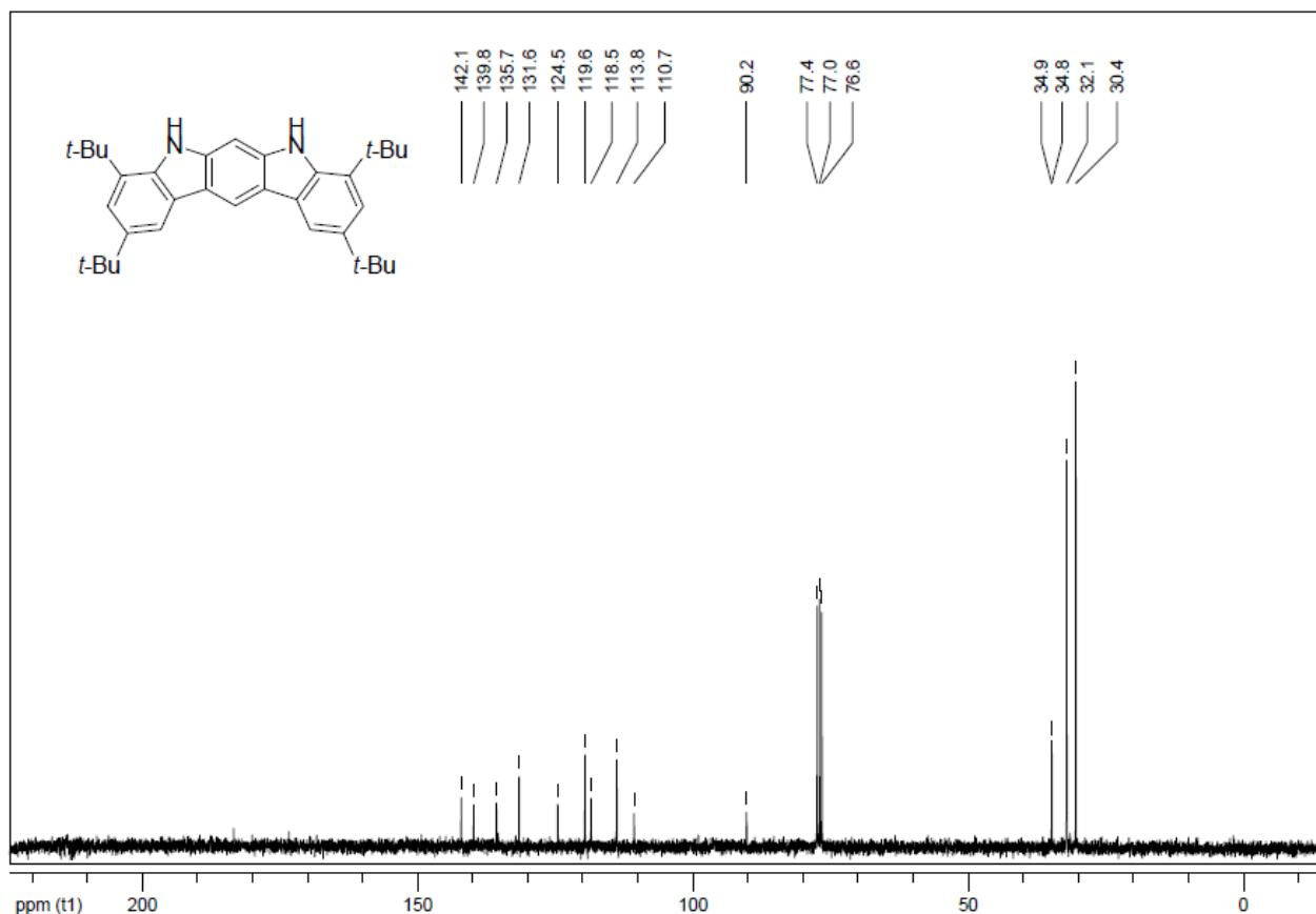
**Fig. S17.**  $^{13}\text{C}$  NMR spectrum of compound **6** ( $\text{CDCl}_3$ , 75 MHz, rt).
