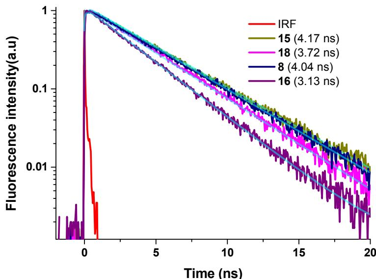
**Fig. S2.** Time-resolved fluorescence decay profiles of **8**, **15**, **16** and **18** in toluene obtained by using TCSPC technique with the photoexcitation at 370 nm with the best fit curves (cyan lines). Temporal profile for instrumental response function is plotted for comparison (red line, fwhm of  $\sim$  30 ps)
