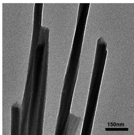
**Figure S5:** TEM images (b-d) of the resultant helical 4-L-HDGA@HKUST-1.
