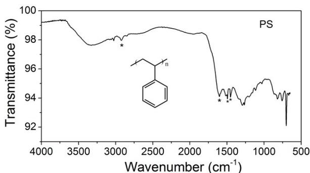
**PS:** The absorption between 2800  $\text{cm}^{-1}$  and 3000  $\text{cm}^{-1}$  are the asymmetric and symmetric stretching vibrations of  $-\text{CH}_2$ . The bands at 1601  $\text{cm}^{-1}$ , 1493  $\text{cm}^{-1}$ , 1452  $\text{cm}^{-1}$  can be assigned to the vibration of the benzene ring.
