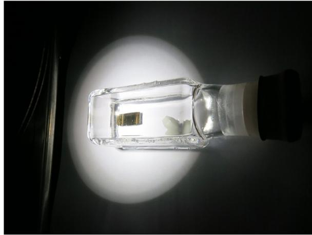
**Fig. S2** Surface-initiated polymerization setup.
