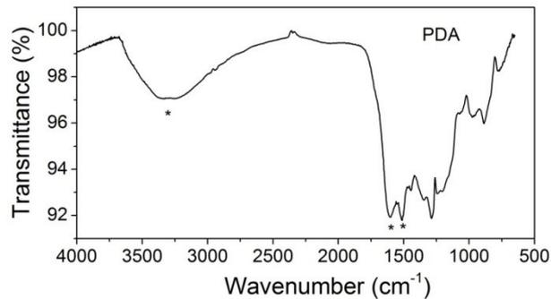
**PDA:** Peaks at 1515 and 1600  $\text{cm}^{-1}$ , an absorption band between 3200-3500  $\text{cm}^{-1}$  (stretching vibration of catechol -OH groups) appeared, supporting the presence of PDA on the gold substrate.
