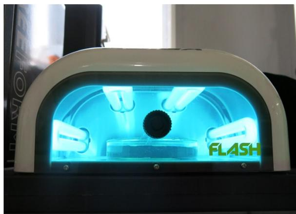
**Fig. S1** Setup for UV assisted deposition of polydopamine.
