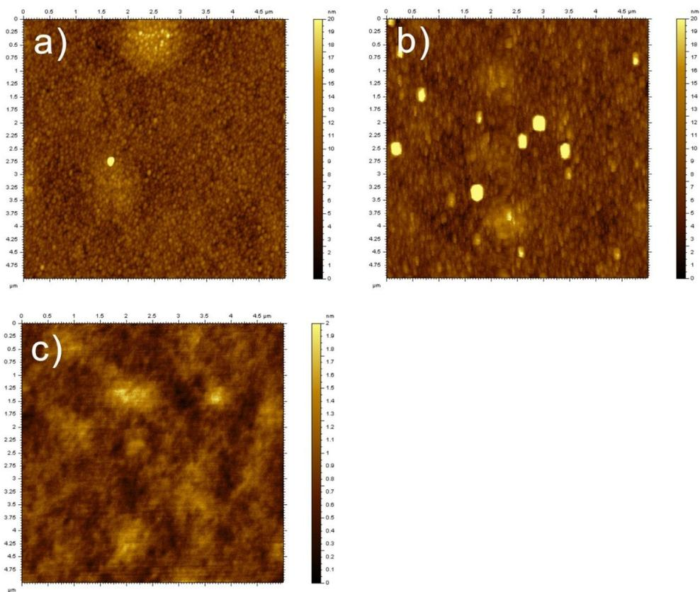
**Fig. S6** Roughness analysis of polydopamine and polymer coatings. The root mean square (RMS) roughness of gold, polydopamine (35 nm) coated gold, and PSPMA (87 nm) coated Au was measured by AFM. The RMS roughness was 2.08 nm for bare Au (a), 2.84 nm for polydopamine coated Au (b), and 0.25 nm for PSPMA coated Au surface (c).
