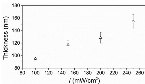
**Fig. S7** PMETAC film thickness as a function of optical intensity ( $I$ ) of the simulated sunlight.
