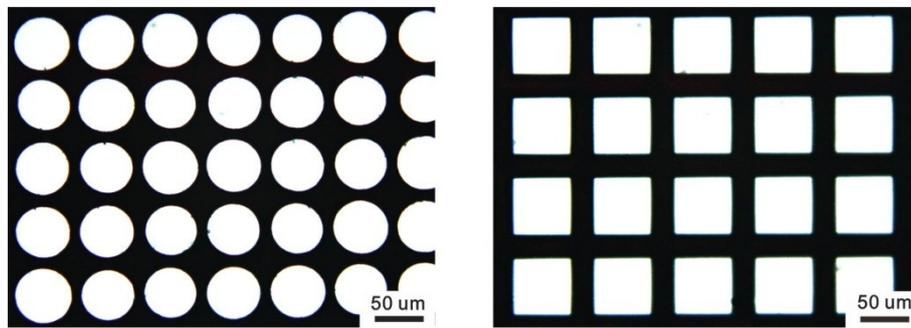
**Fig. S3** Optical microscopy images of two types of photomasks used in this experiment.
