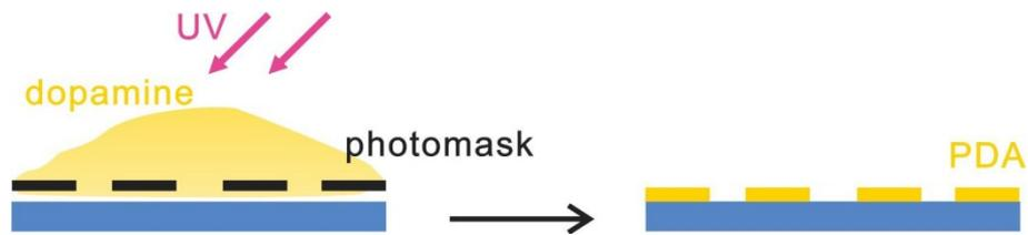
**Fig. S4** Patterning of PDA using a photomask.
