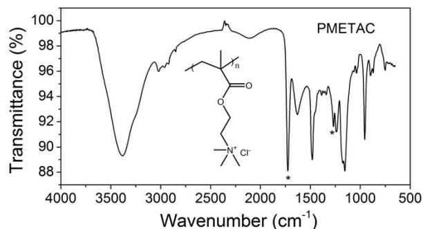
**PMETAC:** The peaks at  $1720\text{ cm}^{-1}$  (C=O stretching) and  $1265\text{ cm}^{-1}$  (C-N stretching) demonstrated the successful grafting of the PMETAC.
