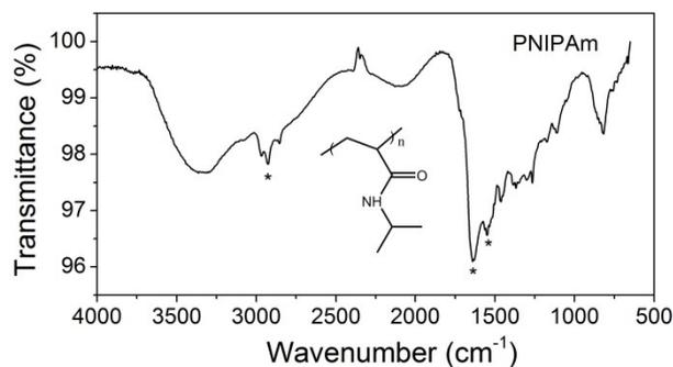
**PNIPAm:** Peaks of the C-H groups (2900-3000  $\text{cm}^{-1}$ ), and the two characteristic peaks at 1640  $\text{cm}^{-1}$  (amide stretch) and 1550  $\text{cm}^{-1}$  (N-H stretch) indicate the success grafting of PNIPAm.
