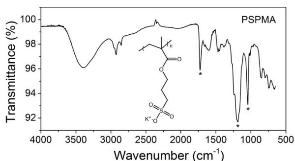
**PSPMA:** The spectra show the stretching of carbonyl groups at  $1730\text{ cm}^{-1}$ , asymmetric sulfonate stretch around  $1200\text{ cm}^{-1}$ , symmetric sulfonate stretching around  $1045\text{ cm}^{-1}$ , and the stretching of C-O in the ester at  $1245\text{ cm}^{-1}$ .
