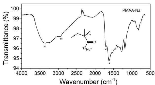
**PMAA-Na:** The strong absorption peak at  $1620\text{ cm}^{-1}$  and  $1700\text{ cm}^{-1}$  should belong to the absorption of carboxylic groups, the appearance of peak between  $3200\text{-}3500\text{ cm}^{-1}$  indicates the presence of -OH. The absorption peaks in the region  $2800\text{-}3000\text{ cm}^{-1}$  correspond to the -CH<sub>2</sub> and -CH<sub>3</sub> groups.
