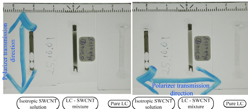
**Supplementary Figure 1.** Three capillaries filled with an isotropic SWCNT suspension, LC-aligned SWCNTs, and CNT-free LC, respectively (left to right), next to each other, underneath a linear polariser held with its transmission direction parallel (left photo) and perpendicular (right photo) to the capillary axes, respectively. Only the sample with LC-aligned SWCNTs changes its appearance, reflecting the alignment of the SWCNTs along the capillary axis.
