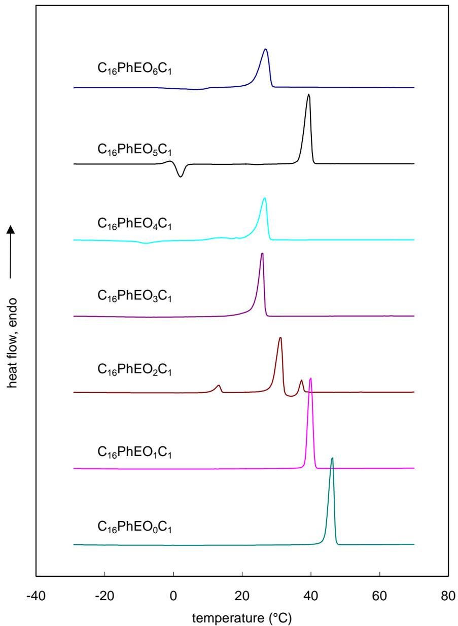
**Figure S-2.** DSC second heating scans of  $C_{16}PhEO_yC_1$  run at  $10^\circ/min$  under a He atmosphere. Samples were held at  $100^\circ C$  for 5 minutes, quenched to  $-100^\circ C$  at rate of  $200^\circ/min$  and held at  $-100^\circ C$  before initiating the heating scan.
