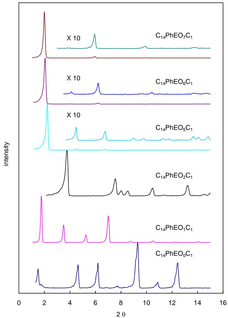
**Figure S-5.** Low angle XRD data for  $C_{14}PhEO_yC_1$ . The samples were cooled from the melt and held at room temperature for 20 h prior to analysis.
