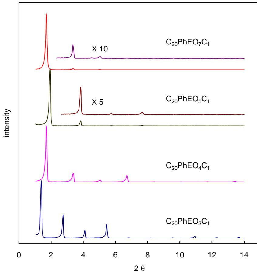
**Figure S-10.** Low angle XRD data for annealed  $C_{20}PhEO_yC_1$ . Prior to analysis, the samples were annealed  $2^\circ$  below their melting point until they reached their ultimate stable structure ( $\sim 2$ - $10$  h).
