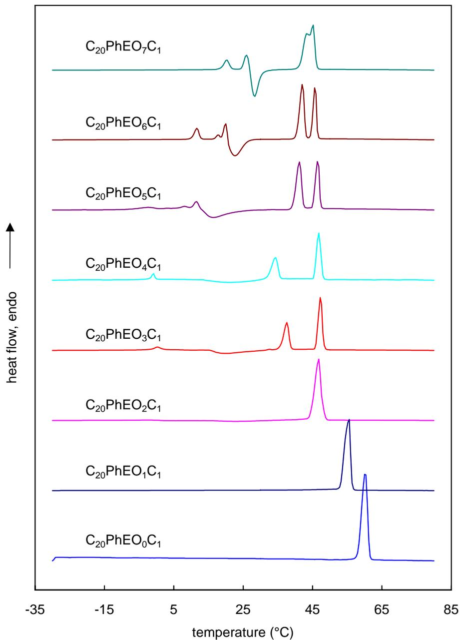
**Figure S-4.** DSC second heating scans of  $C_{20}PhEO_yC_1$  run at  $10\text{ }^\circ\text{/min}$  under a He atmosphere. Samples were held at  $100\text{ }^\circ\text{C}$  for 5 minutes, quenched to  $-100\text{ }^\circ\text{C}$  at rate of  $200\text{ }^\circ\text{/min}$  and held at  $-100\text{ }^\circ\text{C}$  before initiating the heating scan.
