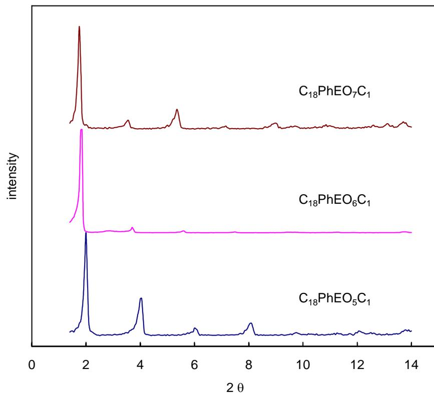
**Figure S-9.** Low angle XRD data for annealed  $C_{18}PhEO_yC_1$ . Prior to analysis, the samples were annealed  $2^\circ$  below their melting point until they reached their ultimate stable structure ( $\sim 2$ -10 h).
