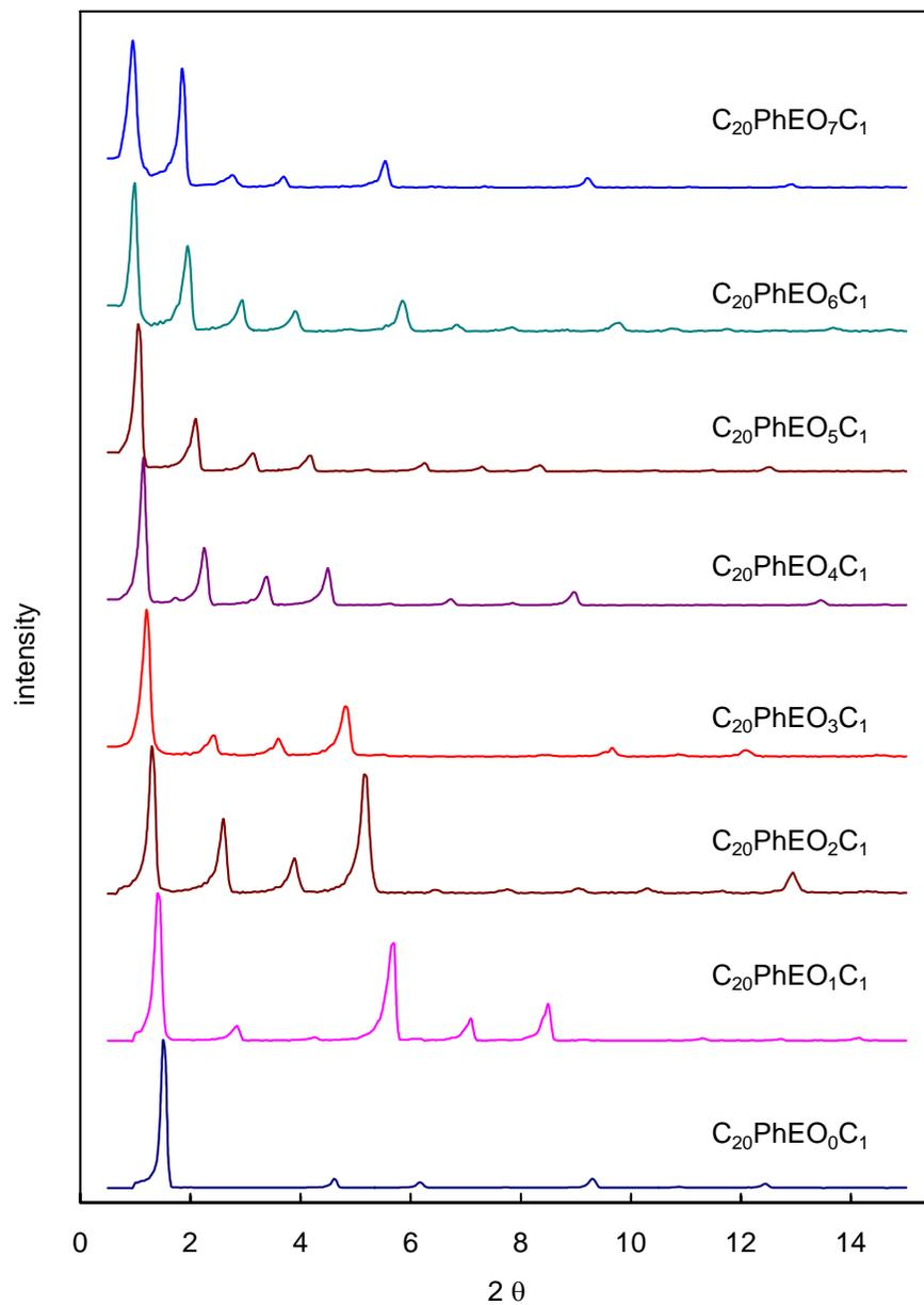
**Figure S-8.** Low angle XRD data for  $C_{20}PhEO_yC_1$ . The samples were cooled from the melt and held at room temperature for 20 h prior to analysis.
