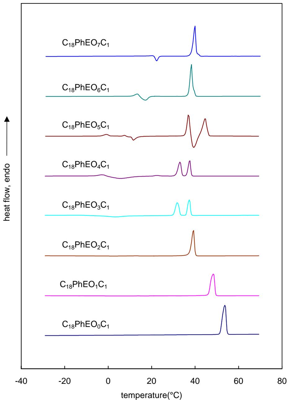
**Figure S-3.** DSC second heating scans of  $C_{18}PhEO_yC_1$  run at 10 °/min under a He atmosphere. Samples were held at 100 °C for 5 minutes, quenched to -100 °C at rate of 200°/min and held at -100 °C before initiating the heating scan.
