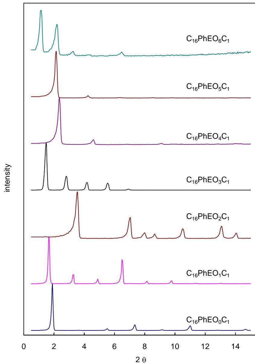
**Figure S-6.** Low angle XRD data for  $C_{16}PhEO_yC_1$ . The samples were cooled from the melt and held at room temperature for 20 h prior to analysis.
