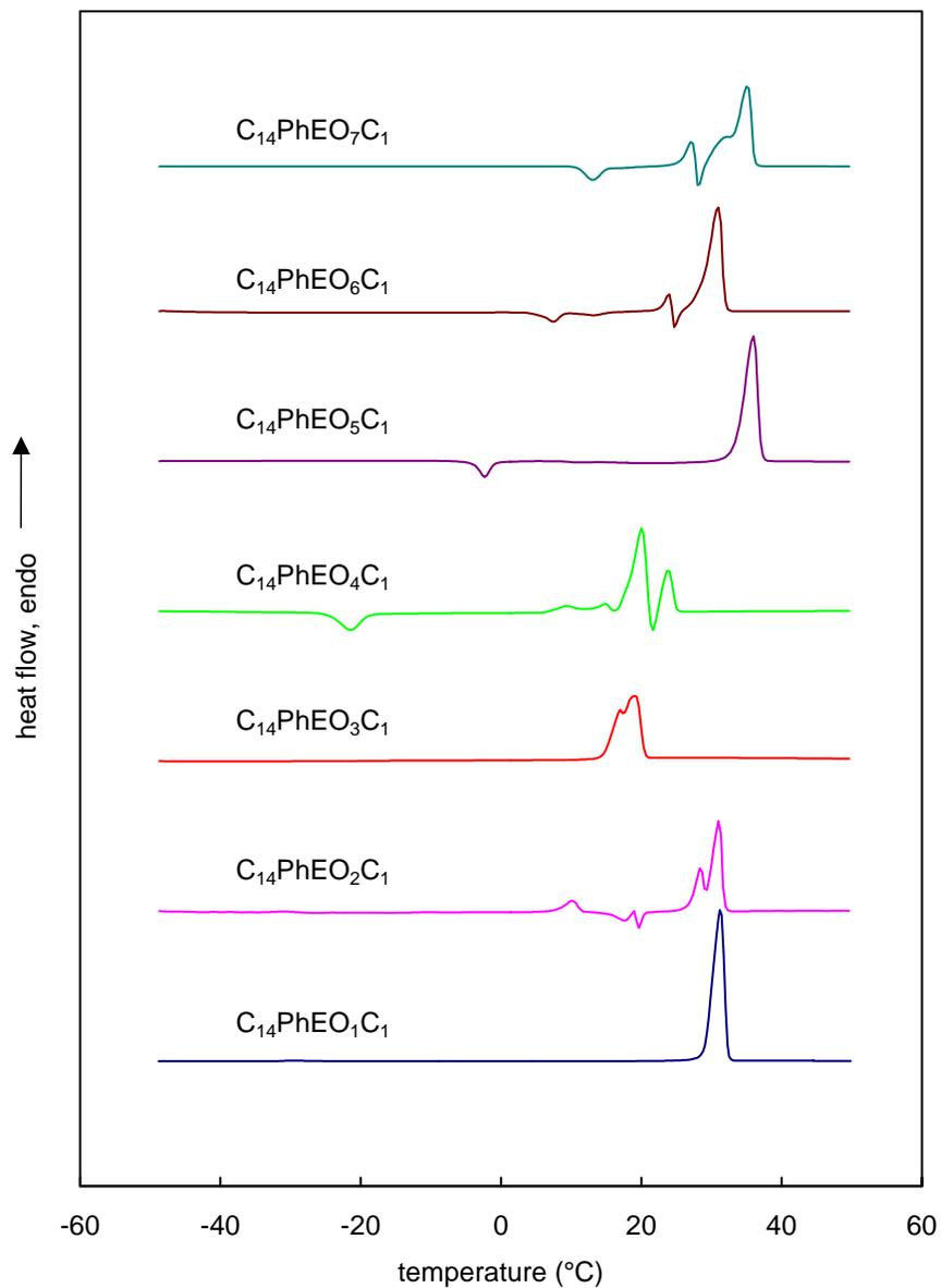
**Figure S-1.** DSC second heating scans of  $C_{14}PhEO_yC_1$  run at 10 °/min under a He atmosphere. Samples were held at 100 °C for 5 minutes, quenched to -100 °C at rate of 200°/min and held at -100 °C before initiating the heating scan.
