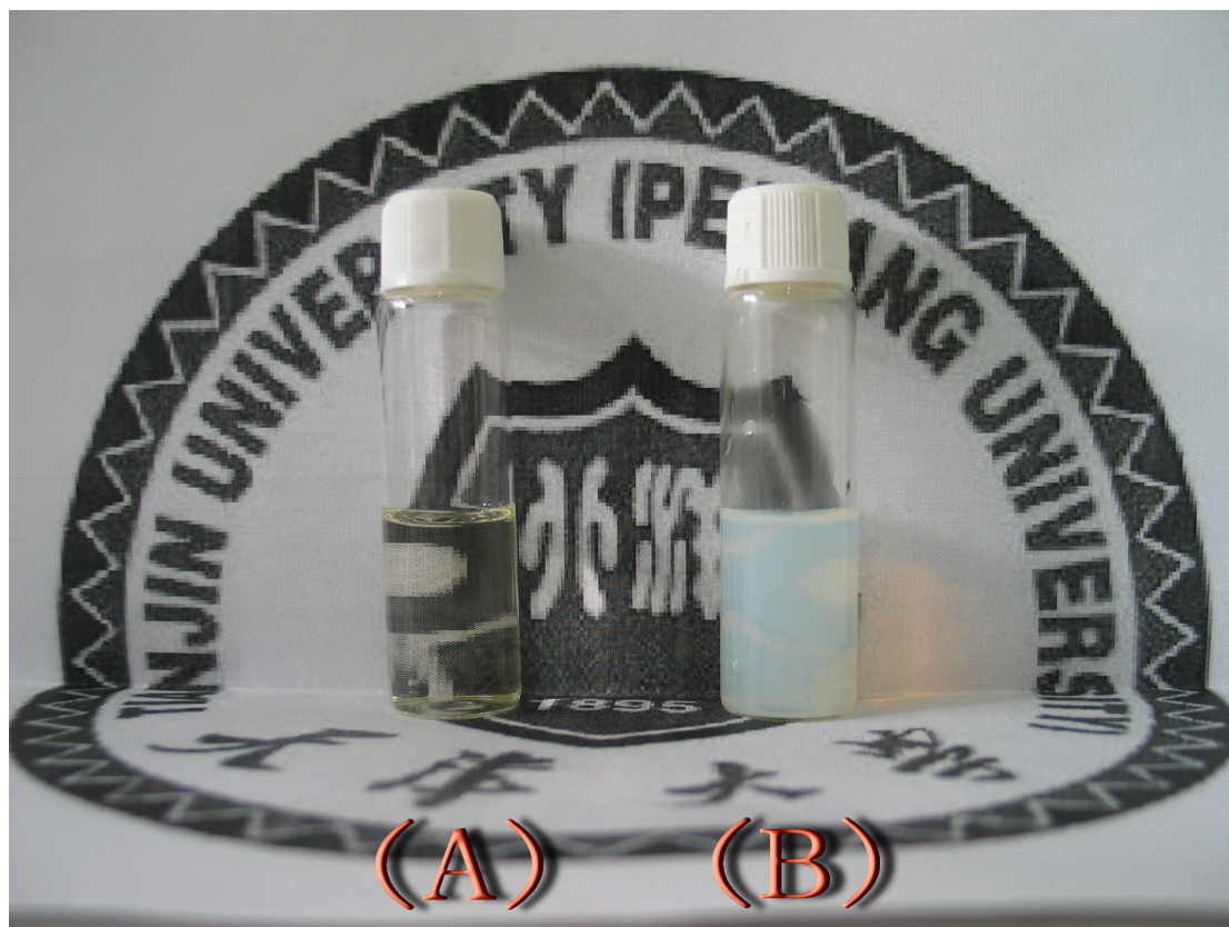
Fig. S3 The typical photographs of thermoresponsive hyperbranched polymers (A) below the LCST, below room temperature (B) above the LCST, 30°C (HPEI10K-IBAm 0.95 at 2 mg/mL)
