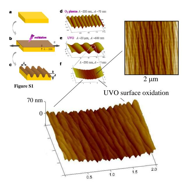
In contrast with oxygen plasma oxidation, UVO induces a complex conversion profile of the top glass-like layer in PDMS which results in secondary ('nested') buckling and comparatively larger dominant wavelengths (10s of  $\mu m$ ).
