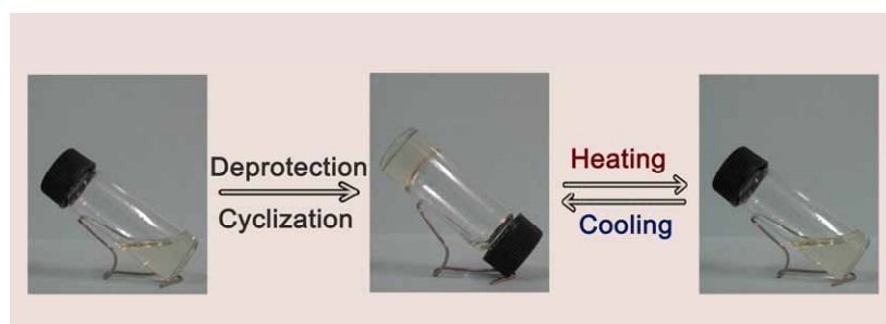
Figure S1 Solution of 25 mg FLF-TM in 1 ml 20 wt% piperidine/DMF (left) and organogel formed in situ upon standing after deprotection and cyclization (middle), which turn to solution when heating (right) and back to gel when cooling.
