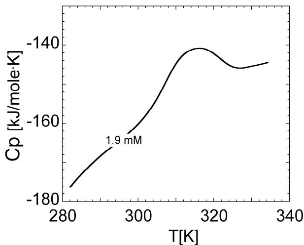
The enthalpy calculated from this thermogram is  $-166 \pm 12$  kJ/mole of protein, which corresponds to  $\Delta H = -250 \pm 20$  kJ/mole triple helix, while the  $\Delta C_p$  maximum occurs at a temperature of  $T_m = 315$  K. These data are in good agreement with literature data for pure (GlyProGly)<sub>9</sub>.<sup>18</sup> If we consider this to be the temperature at which half of the helices have melted (i.e.  $C_H = C_T/3$ ), we can calculate  $K_{H,0}$  from
