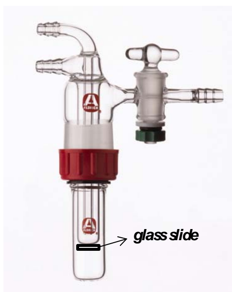
Figure ESI1. Microsublimation apparatus with glass slide.
