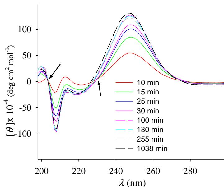
Evolution of the CD spectra at 40 °C, during the tubule formation process, for a 1.2 mM Na-*t*butPhC sample in buffer 30 mM. The arrows show the short time isodichroic points.
