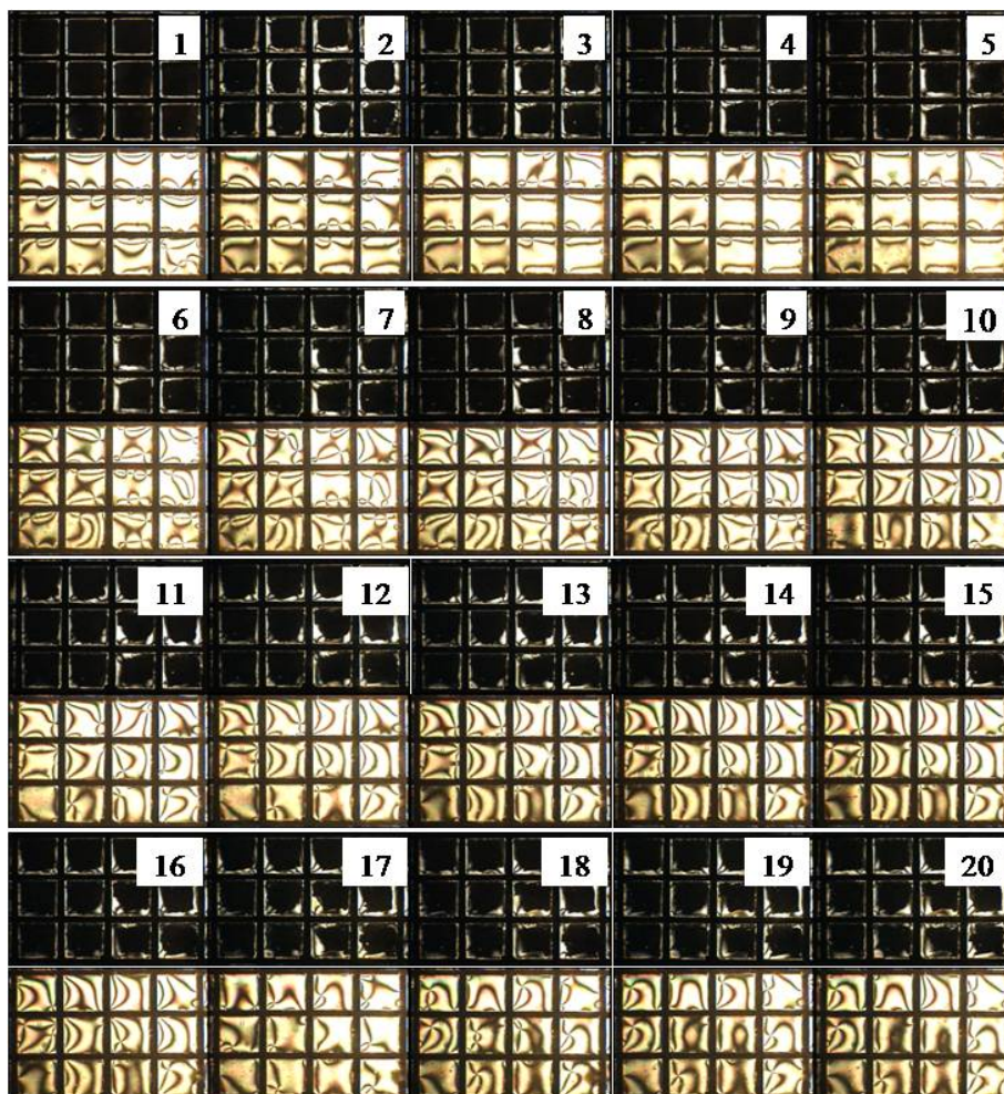
Fig. S7. The optical micrographs of the TEM grid cells during adjustment of the pH in the buffer solution from 12 to 2, 2 to 12, 12 to 2, and 2 to 12, up to 20 cycles after equilibrium; the numbers in the figure indicate cycle.
