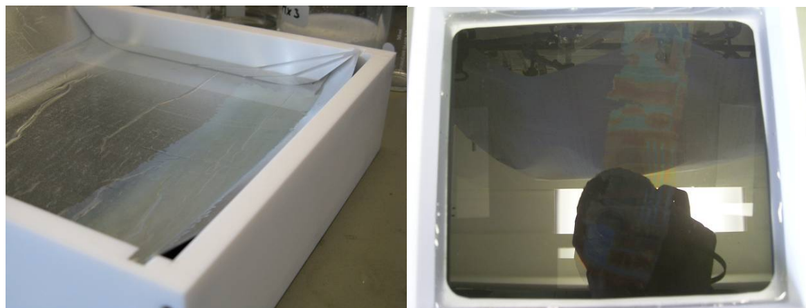
Figure S7. The left side shows a side view with an aluminium foil in place. The right side shows a top view with a floating monolayer (reddish and greenish patches). The black background facilitates visualizing the floating monolayer.
