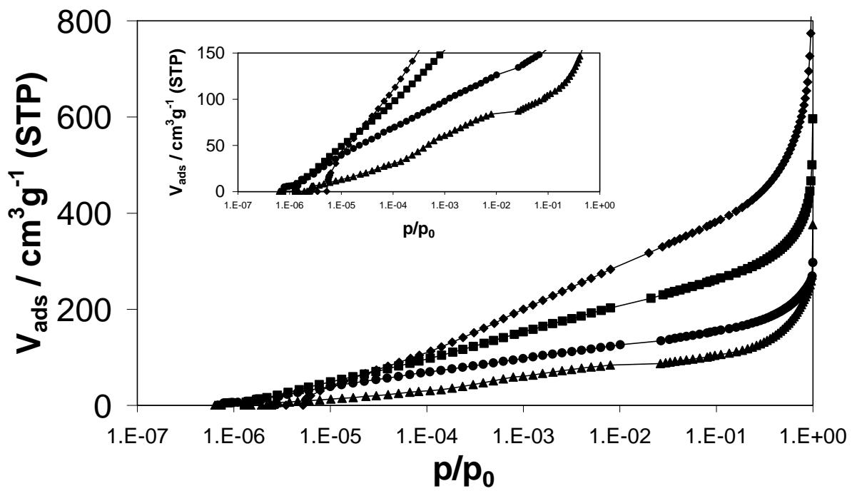
**S7:** Low pressure nitrogen adsorption isotherms of EOF-6 (diamonds), -7 (squares), -8 (triangles), and -9 (circles).
