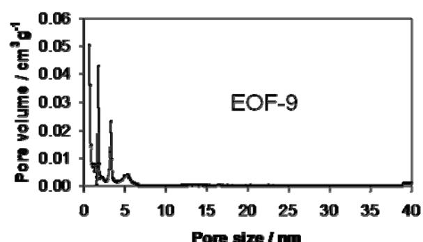
S8: NLDFT pore size distribution for EOF-6 to -9 using N<sub>2</sub> at 77 K on carbon, slit-/cylinder pore, NLDFT eq. model.
