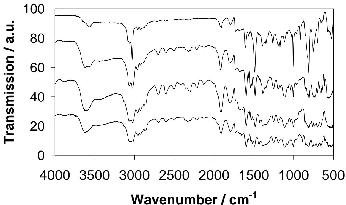
**S6:** FT-IR spectra of EOF-6 (top) to EOF-9 (bottom) measured in diffuse reflection mode.
