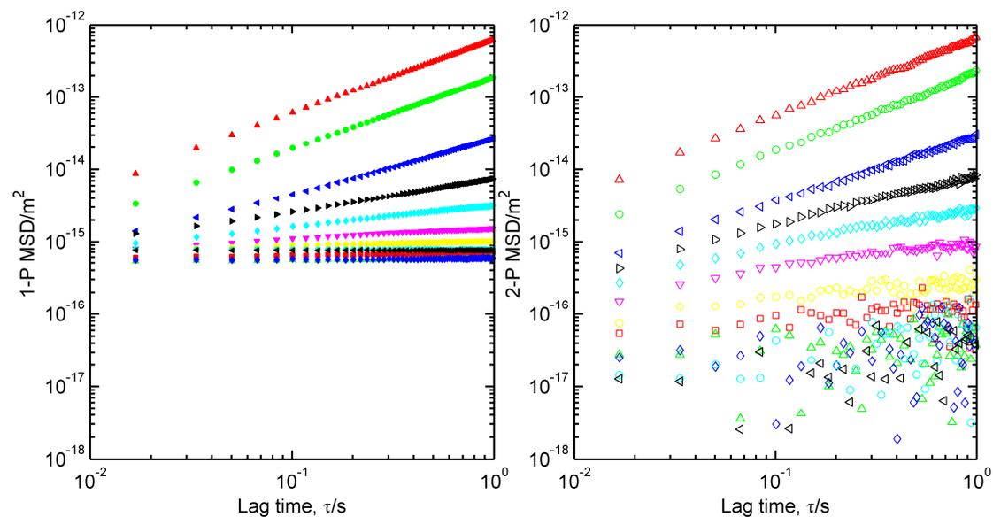
**Fig. S1** Unshifted 1-P (left) and 2-P (right) MSDs for 5% BLG in 50:50 TFE:pH 7 phosphate buffer. Each curve represents a different quasi-static incubation time point. At early times (uppermost curves) there is little difference between 1-P and 2-P MSDs, however the lower limit of the long time 1-P MSDs is limited by the static tracking error, while the 2-P MSDs have no lower bound. The difference in curvature between 1-P and 2-P MSDs is more clearly seen in figure 4 of the main text.
