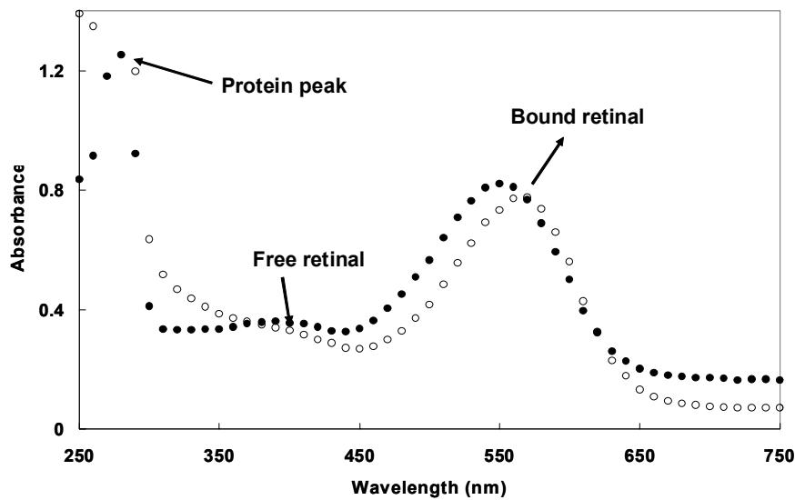
**Figure S1:** The UV-Vis spectra of purple membrane (hollow circles) and bacteriorhodopsin (dissolved in OG, solid circles). The peaks in the range of 250-280nm, 380-420nm and 540-570nm correspond to the presence of total protein (with a contribution from retinal), unbound i.e. free retinal and retinal bound to protein (folded bacteriorhodopsin chromophore), respectively.<sup>7</sup>
