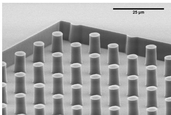
**Figure 1.** SEM micrograph of pillar structure in PE with the corner of the structured area visible. On hexagonal array samples, partial pillars were set into the edge of the area to avoid larger open areas where collapse might occur at a lower pressure.
