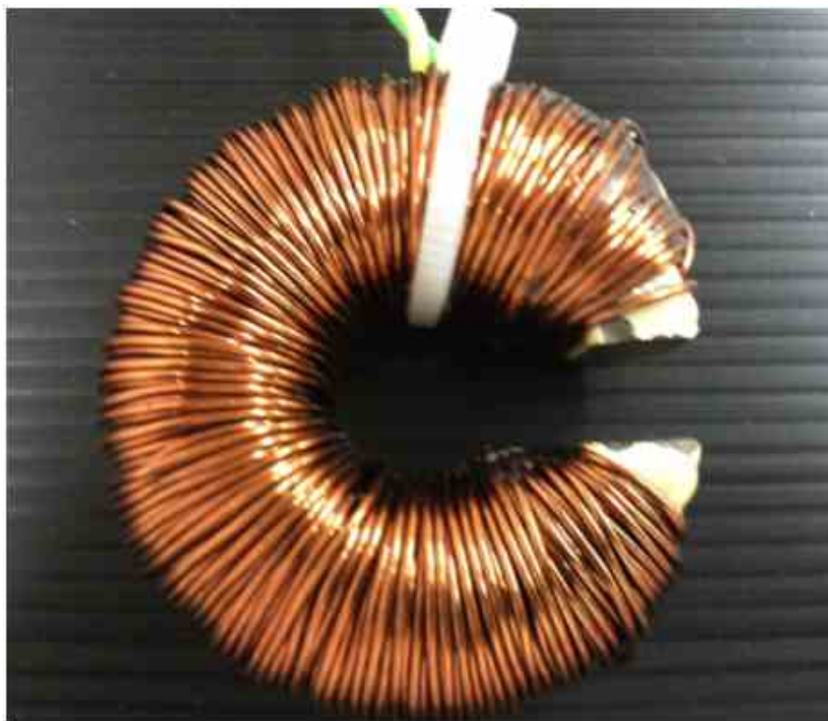
Figure S3. Picture of the broken toroidal magnet used to apply the LF-AMF.
