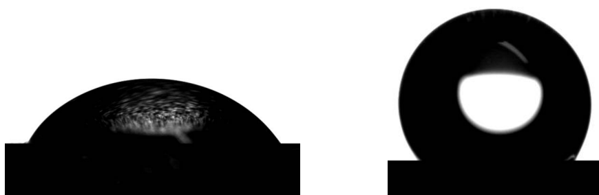
Fig. S3. Advancing contact angle on aluminum alloy plates after standard cleaning procedure (left, 65°) and after treatment with solution of alkoxysilanes in DEPh (right, 130 °, the composition of the mixture is the same as the core of the microcontainers). According to the equation of state derived by Neumann and Li [Li,D., Neumann, A.W., J. Colloid Interface Sci. 1992, 148, 190 ] the surface energy of the aluminum surface after standard procedure of cleaning (contact angle 65°) is equal to 43 mN/m, corresponding value for aluminum surface covered with monolayer of alkoxysilanes (contact angle 130°) is 8 mN/m. This calculations are in a well agreement with [Li,D., Neumann, A.W., J. Colloid Interface Sci. 1992, 148, 190 ]. Standard coatings for aluminum usually demonstrate hydrophilic behavior; contact angles with water usually lie in the range of 50-90 °, which corresponds roughly to the values of surface energy of 54-27 mN/m.
