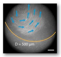
Figure S1: Guidance of molecular motion by micro-patterned surfaces. With circular boundaries (yellow line) persistent swirling motions can be induced as exemplified with a time overlay of 10 consecutive images. The blue arrows mark the margin of the active region and the scale bar is 50  $\mu$ m and the density is set to  $\rho = 18 \mu m^{-2}$ .
