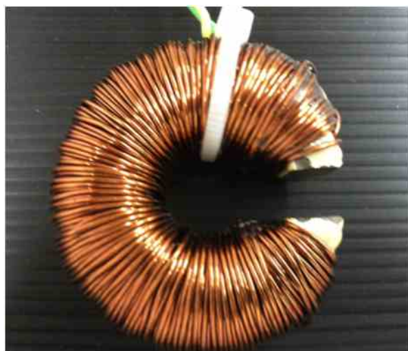
Figure S1. Picture of the broken toroidal magnet used to apply the LF-AMF.
