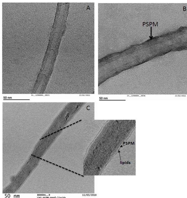
**Fig. S1.** TEM images of modified CNT stained with Sodium Tungstate: oxidised CNTs (A), PSPM coated CNTs (B) and lipid coated CNTs (C)
