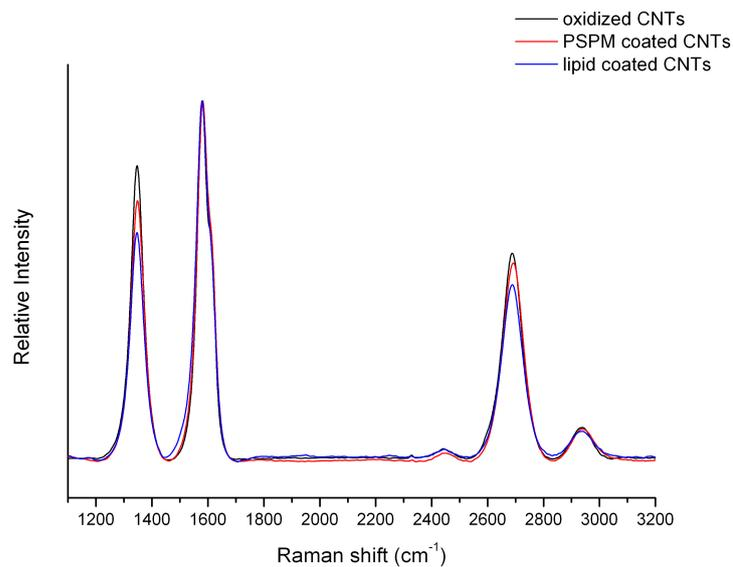
**Fig. S2.** Raman spectra of different surface modified carbon nanotubes.
