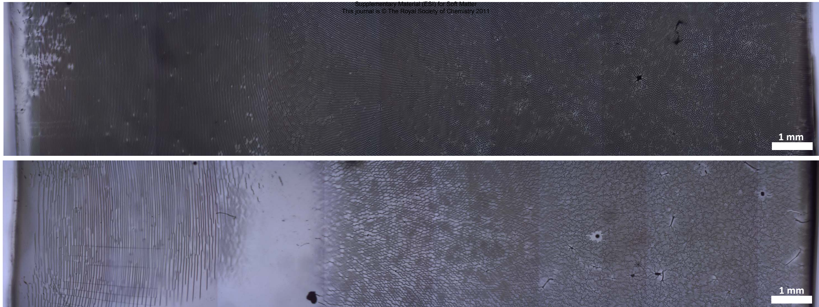
Figure S3: Stitched images depicting the morphological transitions of wrinkled beams across varying states of prestrain. Prestrain is induced by clamping the left ends of the beams during oxidation. a) Beam treated with UVO for 30 minutes, exhibiting the labyrinth morphology on the unclamped end. b) Beam treated with UVO for 20 minutes, resulting in a coalesced dimple morphology on the unclamped end. Dark spots represent dust particles adhered to the PDMS. The observed morphology on the unclamped end of b) is noted to differ from the pure dimples observed in Figure 1; this is likely due to differences in UVO process between the two experiments, including effects resulting from the presence of the clamp as well as differences in the age of the UV bulb.
