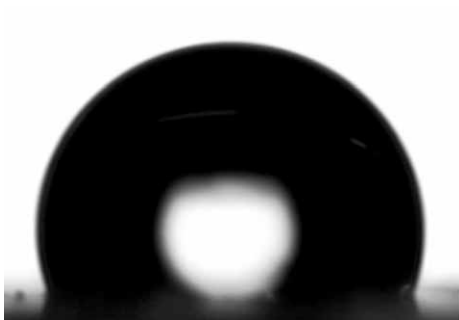
Figure S3. Droplet CA image of flat PDMS. The CA of flat PDMS is 110.2 \pm 1.4^\circ .
