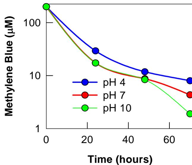
**Figure S2.** Separation of the cationic dye, methylene blue (MB), from buffered solutions of different pH by a laponite-crosslinked NIPA gel. Plots of dye concentration vs. time are shown for three different pH values. The results are nearly identical, indicating that the binding of MB to laponite is unaffected by pH.
