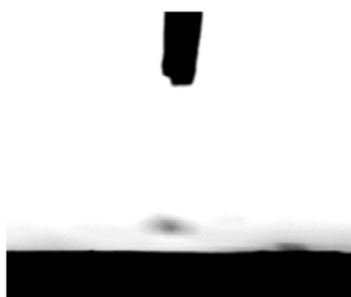
Figure S2. The lower side of lotus leaf shows superhydrophilic property with contact angle almost 0^\circ in air.
