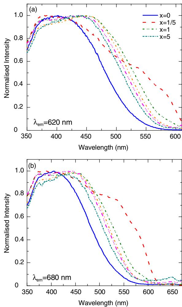
**Fig. s5.** Photoexcitation spectra of P3ImiHT-D<sub>2</sub>O (solid blue lines) and P3ImiHT(SDS) $_x$ -D<sub>2</sub>O  $x=1/5$  (dashed red lines),  $x=2/3$  (dashed and dotted orange lines),  $x=1$  (dashed and double dotted green lines),  $x=3/2$  (dashed and triple dotted magenta lines) for  $x=5$  (double dashed and dotted cyan lines). (a)  $\lambda_{\text{em}}=620 \text{ nm}$ . (b)  $\lambda_{\text{em}}=680 \text{ nm}$ . The overall concentration of all samples was ~0.01 mg/mL.
