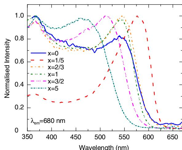
**Fig. s2.** Photoexcitation spectra of P3ImiHT-D<sub>2</sub>O (solid blue line) and P3ImiHT(SDS)<sub>x</sub>-D<sub>2</sub>O  $x=1/5$  (dashed red line),  $x=2/3$  (dashed and dotted orange line),  $x=1$  (dashed and double dotted green line),  $x=3/2$  (dashed and triple dotted magenta line) for  $x=5$  (double dashed and dotted cyan line).  $\lambda_{\text{em}}=680 \text{ nm}$ . The overall concentration of all samples was  $\sim 10 \text{ mg/mL}$ .
