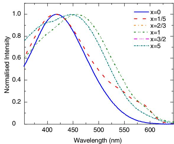
**Fig. s3.** UV/vis spectra of P3ImiHT-D<sub>2</sub>O (solid blue line) and P3ImiHT(SDS) $_x$ -D<sub>2</sub>O  $x=1/5$  (dashed red line),  $x=2/3$  (dashed and dotted orange line),  $x=1$  (dashed and double dotted green line),  $x=3/2$  (dashed and triple dotted magenta line) for  $x=5$  (double dashed and dotted cyan line). The overall concentration of all samples was ~0.01 mg/mL.
