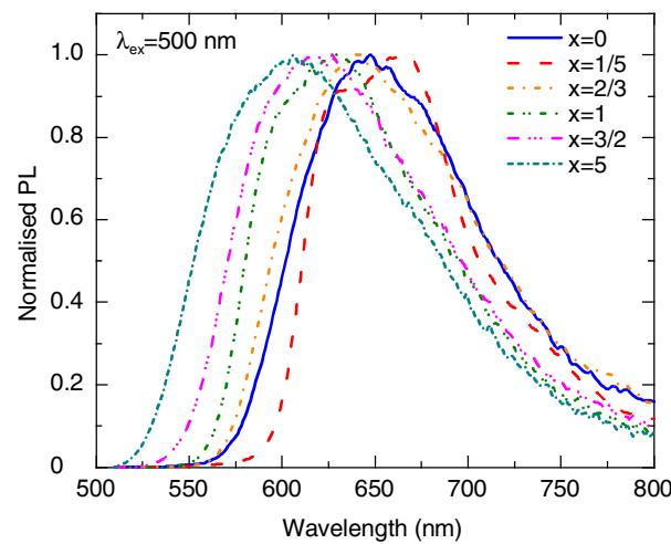
**Fig. s1.** PL spectra of P3ImiHT-D<sub>2</sub>O (solid blue lines) and P3ImiHT(SDS) $_x$ -D<sub>2</sub>O  $x=1/5$  (dashed red line),  $x=2/3$  (dashed and dotted orange line),  $x=1$  (dashed and double dotted green line),  $x=3/2$  (dashed and triple dotted magenta line) for  $x=5$  (double dashed and dotted cyan line).  $\lambda_{\text{ex.}}=500$  nm.
