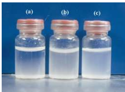
Fig. S1 The photographs for the dispersion of the ungrafted MIP (a), B-MIP-12h (b), and H-MIP-12h (c) microspheres in pure water (1 mg/mL) at 20 °C (after settling down for 2 h).
