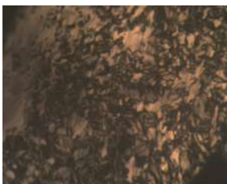
Figure S3. Optical micrographs of 80 wt% [C 14 -Im-3OEG][Cl] in water between Crossed polarizing filters
