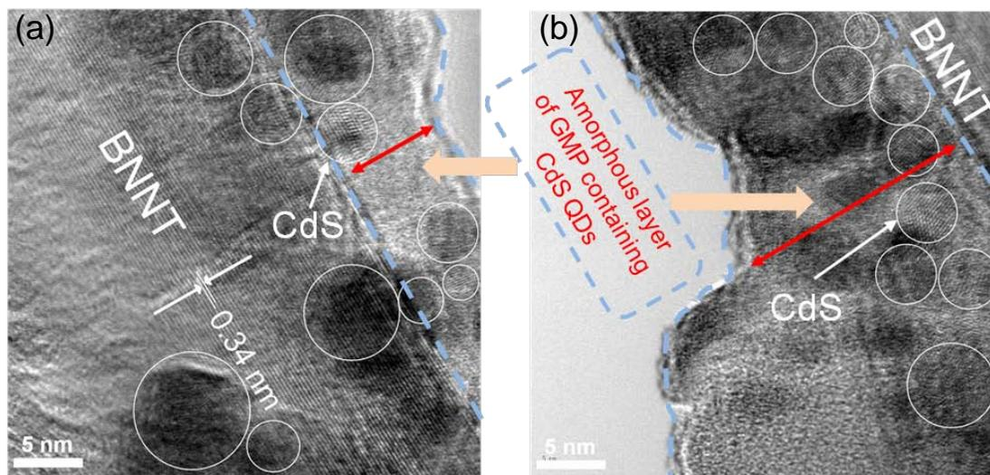
**Fig. S6** (a,b) High-resolution TEM images of CdS/GMP@BNNT hybrids. Crystalline CdS QDs were observed on the sidewalls of multiwalled BNNTs (encircled areas).
