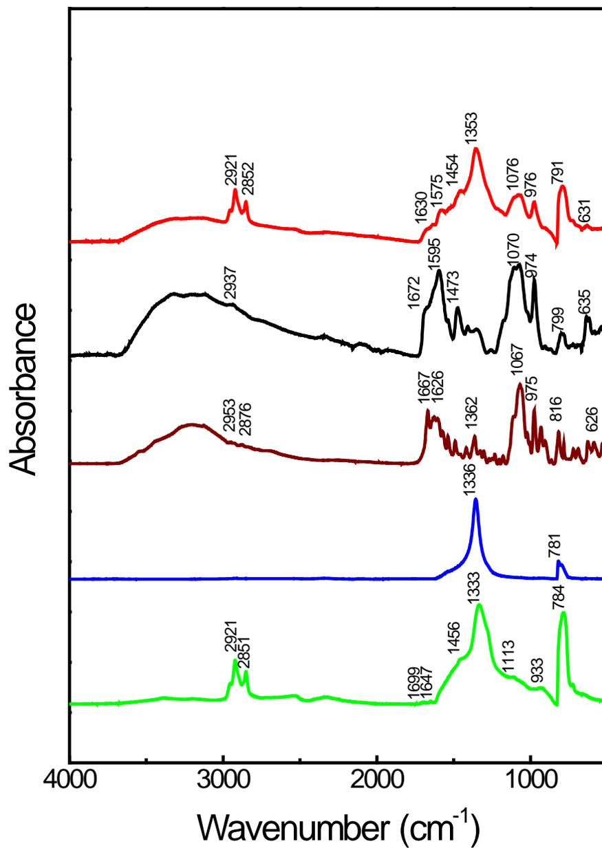
**Fig. S3** FT-IR spectra of CdS/GMP@BNNT hybrids (red), GMP-capped CdS QDs (black), pure GMP (wine), the original BNNTs (blue), and GMP-modified BNNTs (green).
