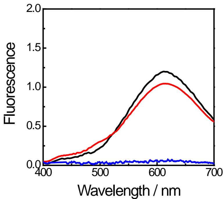
**Fig. S9** Comparative fluorescence spectra of as-prepared GMP-capped CdS QDs (black), the QDs solution after sonication for 3 h (red), and the QDs solution after sonication for 3 h, incubation for 24 h, and purification processes, similarly with CdS/GMP@BNNT hybrids (blue).
