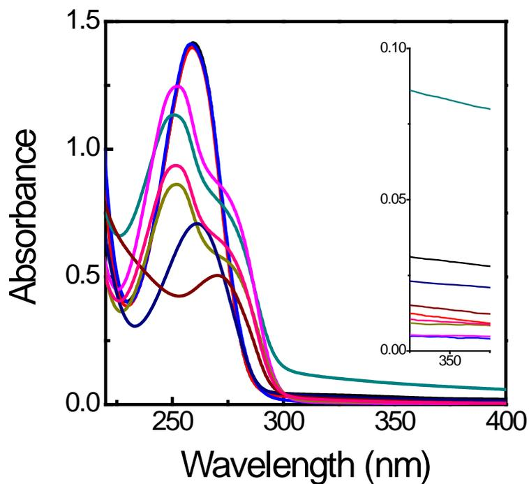
**Fig. S2** UV-vis absorption spectra of nucleotides-modified BNNTs. AMP-modified BNNTs (black), ADP-modified BNNTs (red), ATP-modified BNNTs (blue), GMP-modified BNNTs (dark cyan), GDP-modified BNNTs (magenta), GTP-modified BNNTs (dark yellow), UMP-modified BNNTs (navy), CMP-modified BNNTs (wine), and Gua-modified BNNTs (pink). The inset shows an enlarged part from 345 nm to 355 nm.
