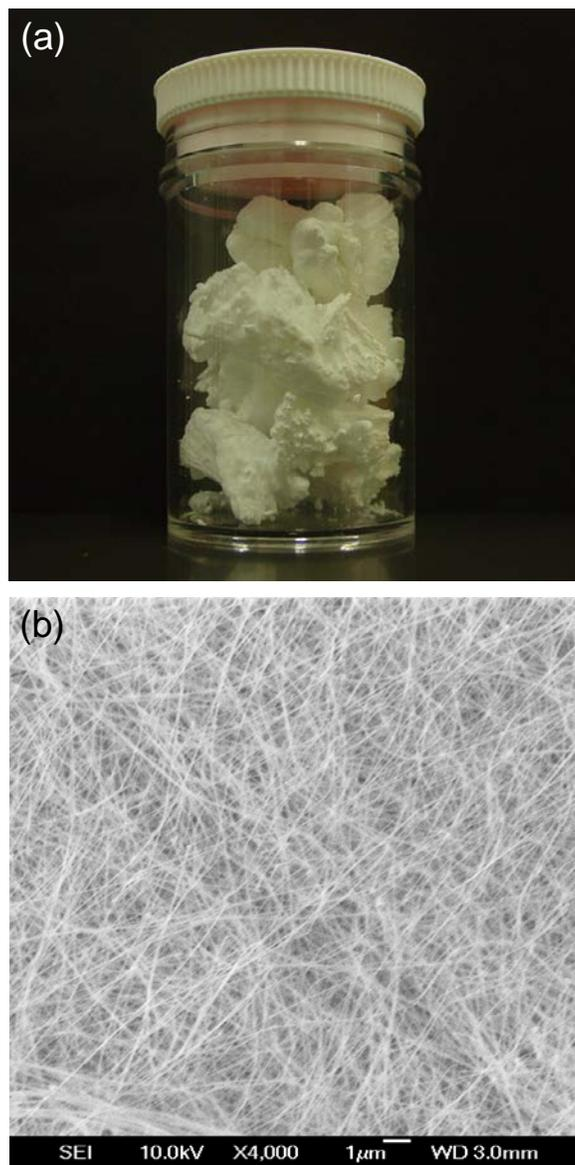
**Fig. S1** (a) Typical photograph and (b) SEM image of pristine BNNTs.
