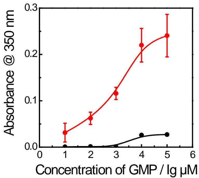
**Fig. S4** Dependence of the dispersed amounts of BNNTs (red) on the concentration of GMP, and absorption of GMP solution (black).
