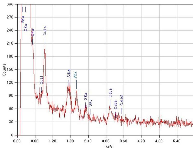
**Fig. S7** EDS data of CdS/GMP@BNNT hybrids. The peak of PKa suggests the presence of GMP in the hybrids, and the peaks of SKa, SKb, CdLa, CdLb, and CdLb2 suggest the presence of CdS in the hybrids.
