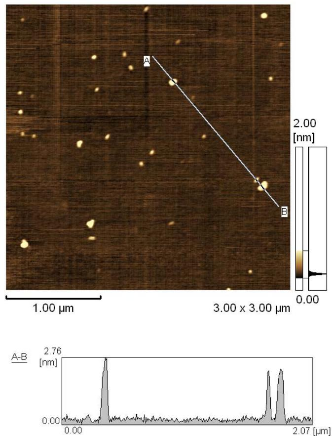
**Fig. S10** AFM image and height profile of GMP-capped CdS QDs after sonication for 3 h. Compared with as-prepared QDs (see Fig. S4 for AFM image), the morphological features were almost similar, suggesting that the sonication procedure does not notably affect the QDs.
