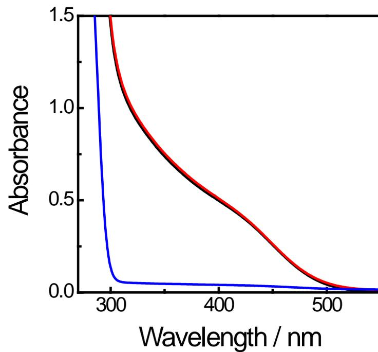
**Fig. S8** Comparative UV-vis spectra of as-prepared GMP-capped CdS QDs (black), the QDs solution after sonication for 3 h (red), and the QDs solution after sonication for 3 h, incubation for 24 h, and purification processes, similarly with CdS/GMP@BNNT hybrids (blue).
