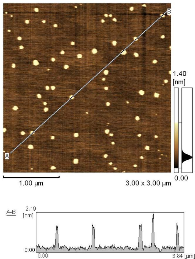
**Fig. S5** AFM image and height profile of as-prepared GMP-capped CdS QDs. Most QDs have sizes around 2 nm. A small number of QDs have sizes around 8 nm.
