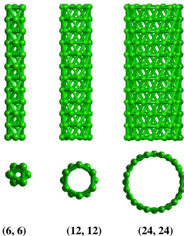
Figure S1. Side (top) and top (bottom) views of coarse-grained structures of SWNTs used in the simulations.
