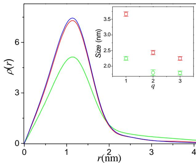
Figure S4. The radial density profiles for the PE chains grafting on the (12, 12) SWNT with various valencies of the counterions from added salt: (green)  $q=1$ , (red)  $q=2$  and (blue)  $q=3$ . The inset shows the thickness,  $L_c$ , (red) and the radius of gyration,  $R$ , (green) of the PE chains as a function of the counterion valency. The graft density of PE chains is  $\alpha = 0.008$ .
