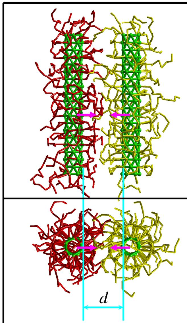
Figure S7. The side (top) and top (bottom) views of the configuration for two grafted SWNTs in the calculation of PMF. Color scheme: (green) bonds and beads of SWNT, (red) PE chains on the left SWNT and (yellow) PE chains on the right SWNT. Water and other ions are not shown for clarity. The pink arrows represent the moving direction of the SWNTs.
