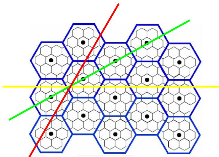
Figure S5. Schematic representation of the pitch angle threadlines of an armchair SWNT by grouping 24 carbon atoms. Solid dots represent the lumped beads while the thin black lines indicate the carbon-carbon bonds in the SWNT. The red and green lines denote the pitch angle threadlines of the atomistic and the coarse-grained models, respectively. The yellow line is the axis of the SWNT.
