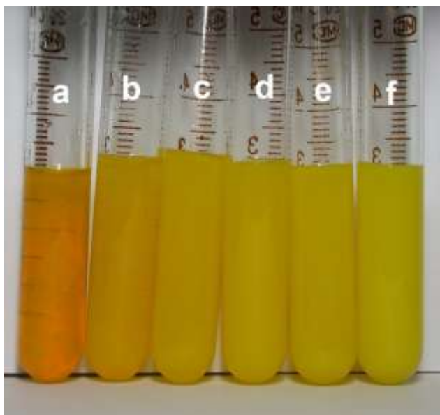
Fig. S1 Pictures of gels (1% w/v) at different methanol content: (a) 0%; (b) 5%; (c) 10%; (d) 15%; (e) 20%; (f) 30%.
