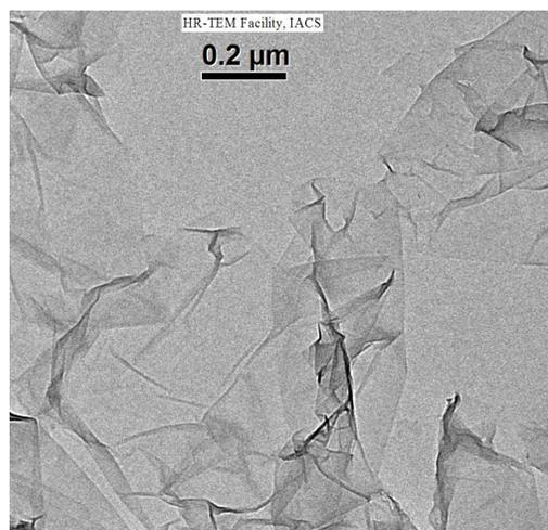
**Fig. S3** Transmission electron microscopic image of reduced graphene oxide (RGO) by ascorbic acid.
