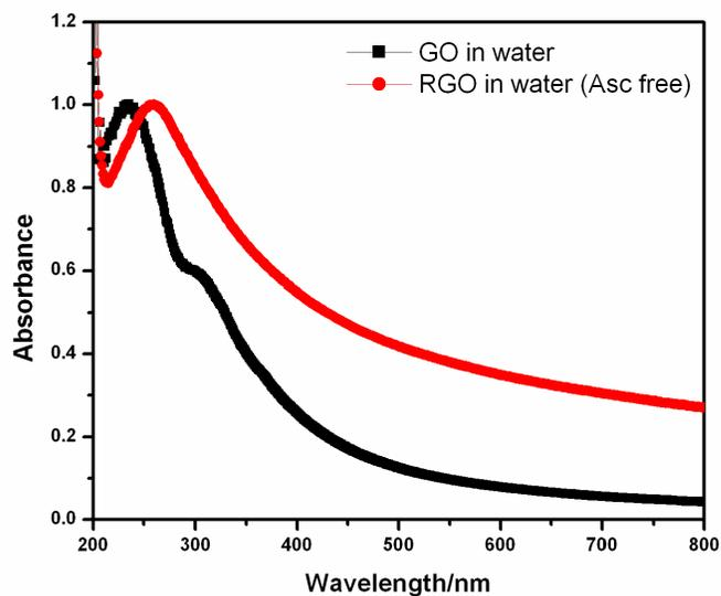
**Fig. S1** UV-Vis spectra during the reduction of graphene oxide (GO) to reduced graphene oxide (RGO).
