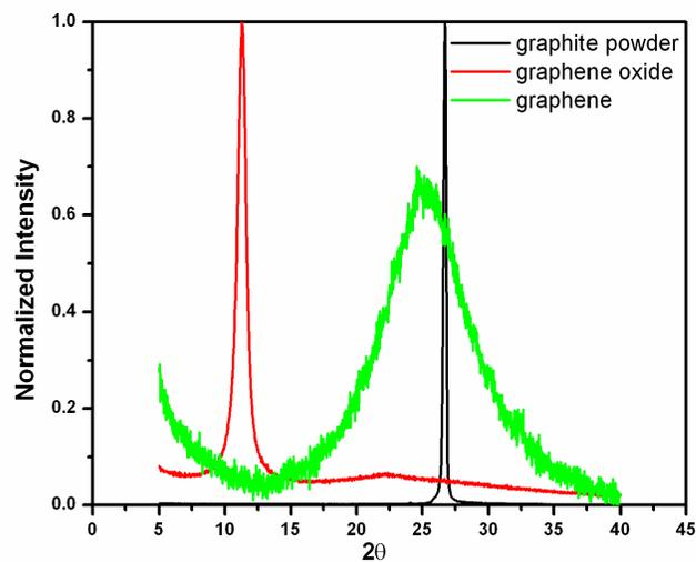
**Fig. S2** X-ray diffraction patterns during the preparation of graphite powder to graphene oxide (GO) to graphene (RGO).
