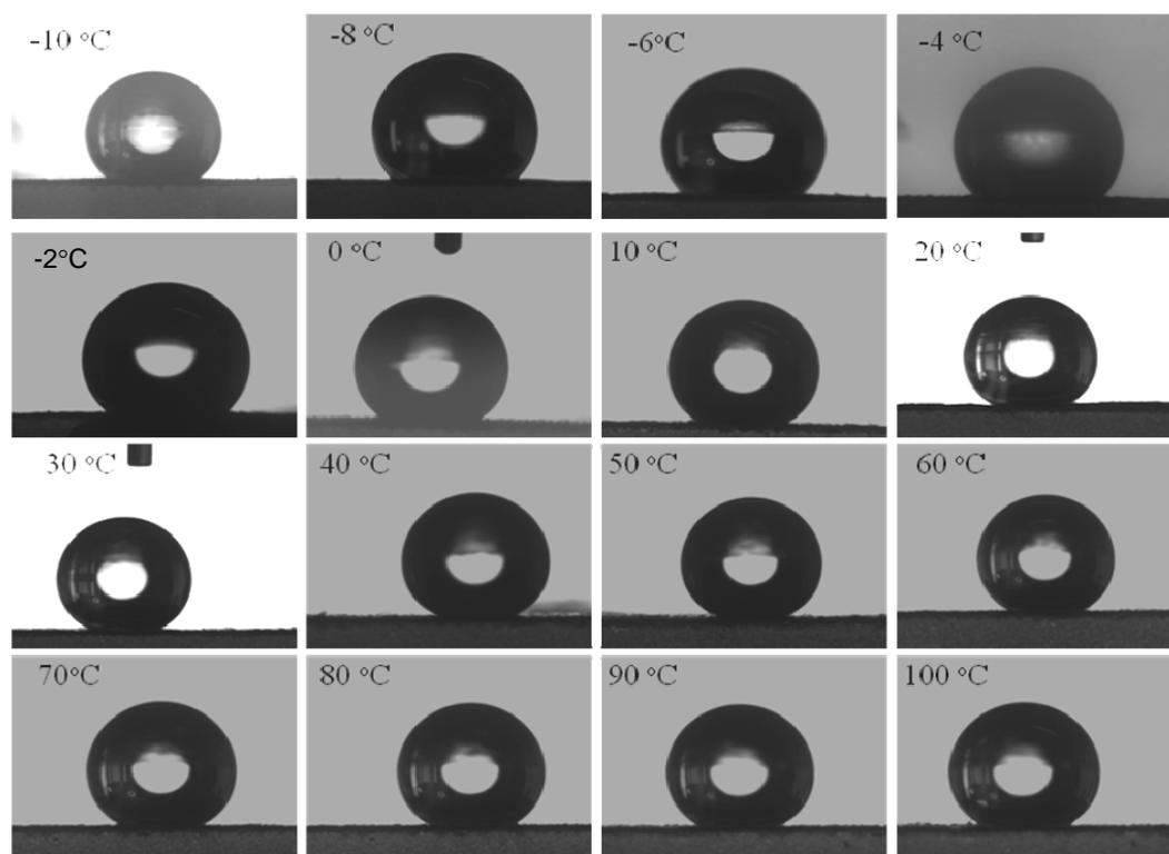
**Figure S3.** Profiles of drops on butterfly wings under temperature changed from 100°C to -10°C, at intermediate relative humidity of 40%. The drops are suspended and the tiny water condensed drops are not distinctly observed on the surfaces.
