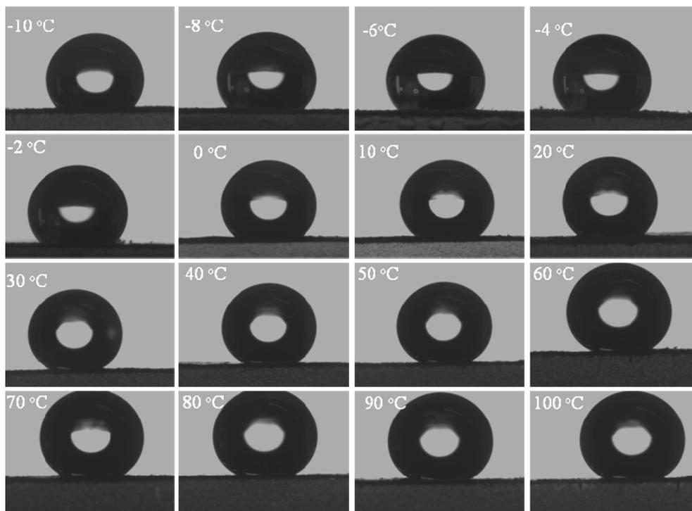
**Figure S4.** Profiles of drops on butterfly wings under temperature changed from  $-7^{\circ}\text{C}$  to  $100^{\circ}\text{C}$  in high relative humidity of  $> 90\%$ . The drops collapse and the tiny condensed drops are observed on the surfaces in the temperature below zero.
