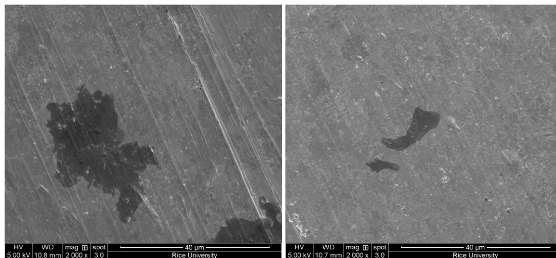
Figure S1: SEM image of GGO flakes showing their irregular, polygonal shape and presence of few ribbon-like structures.
